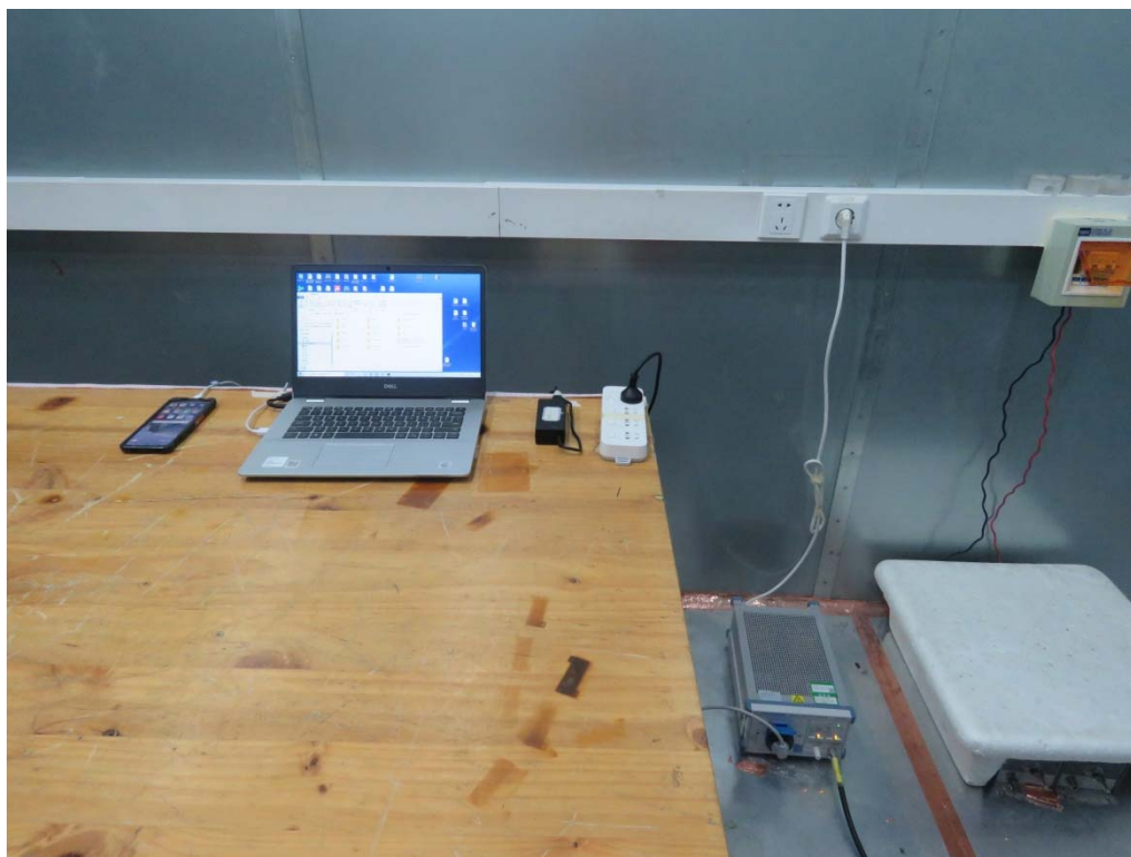
Picture 1: Conducted Emissions Test Setup
