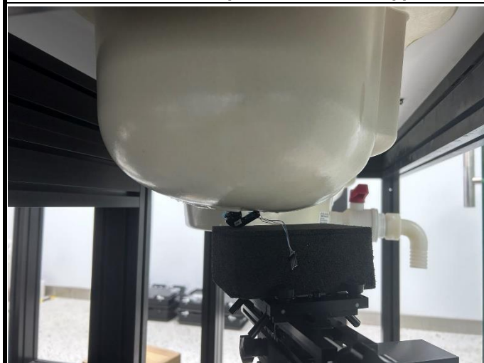
Right Cheek (EUT with 0 cm Gap)
