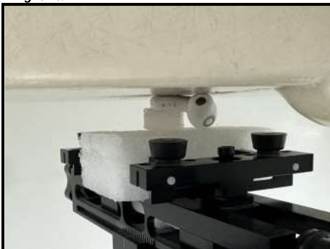
Test Position 1 (EUT with 0 cm Gap)
