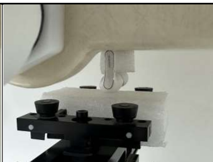
Test Position 6 (EUT with 0 cm Gap)
