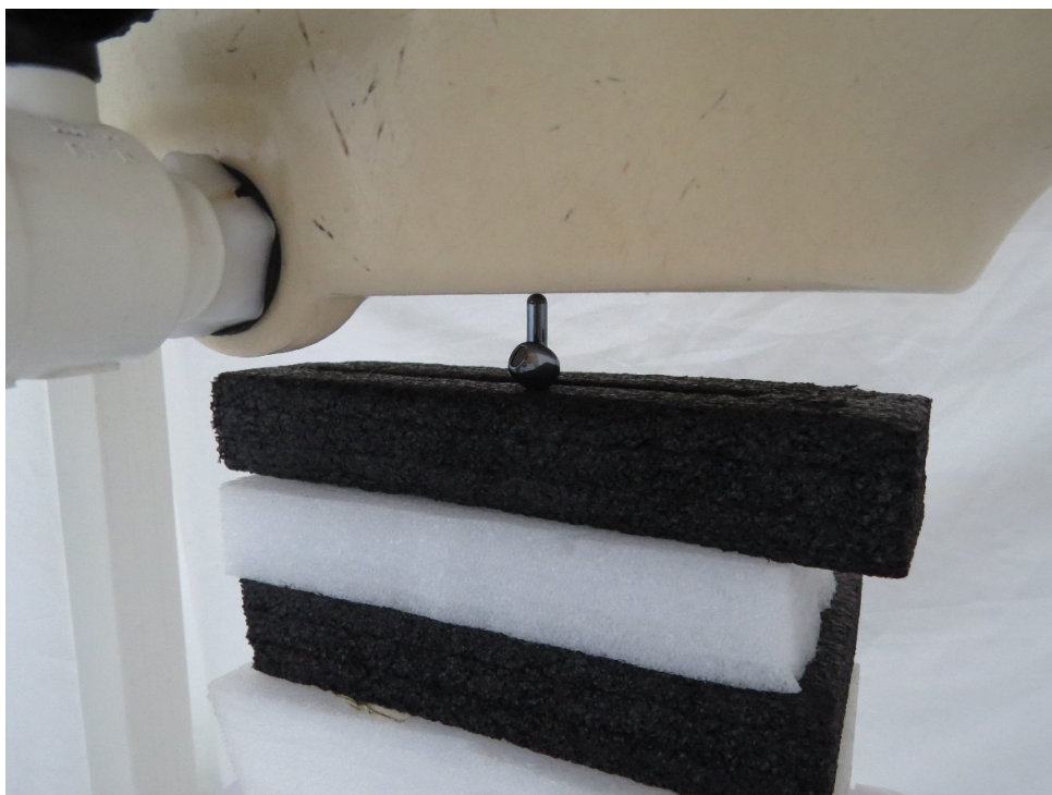
Picture 18: Bottom Edge, the distance from EUT to the bottom of the Phantom is 0mm
