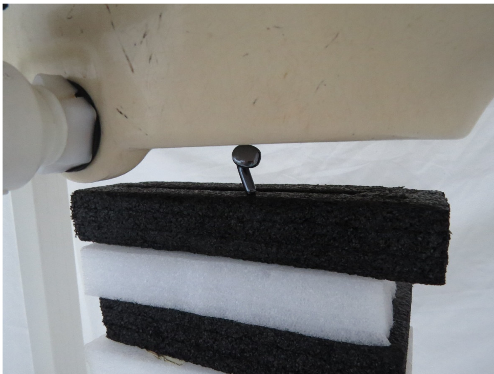
Picture 17: Top Edge, the distance from EUT to the bottom of the Phantom is 0mm
