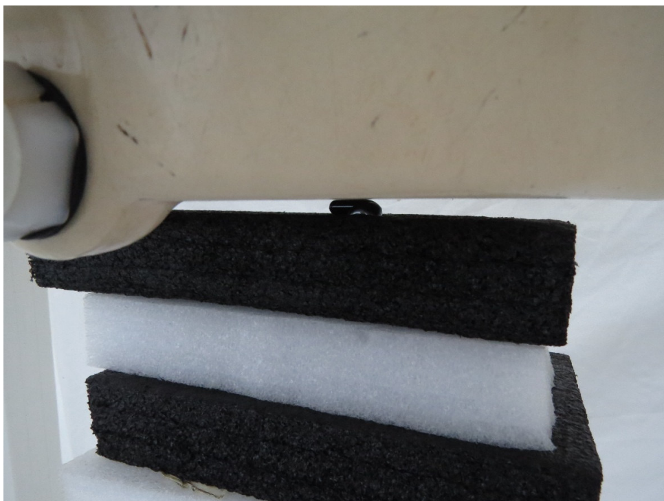
Picture 16: Right Edge, the distance from EUT to the bottom of the Phantom is 0mm
