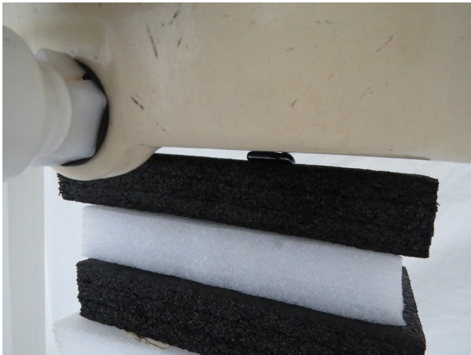
Picture 15: Left Edge, the distance from EUT to the bottom of the Phantom is 0mm
