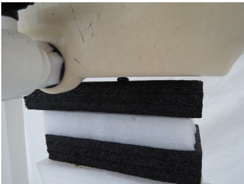
Picture 14: Front Side, the distance from EUT to the bottom of the Phantom is 0mm
