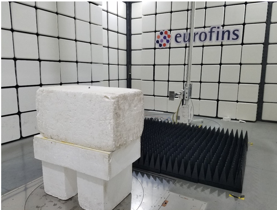
Picture 1 Radiated Emission Test Setup
