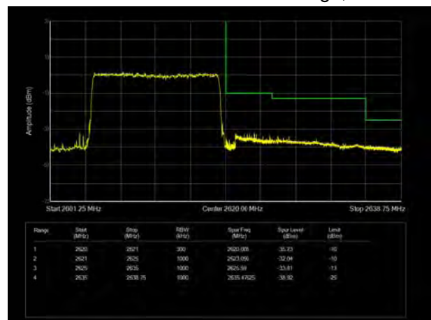
LTE Band 38 16QAM 20MHz CH-High, 1 RB
