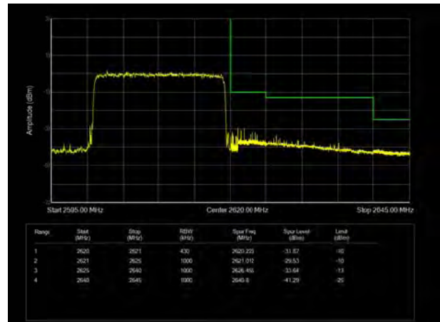
LTE Band 38 64QAM 20MHz CH-High, 100%RB
