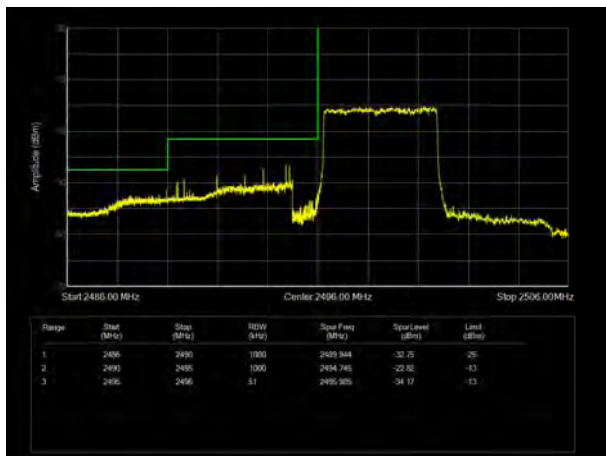
LTE Band 41 QPSK 10MHz CH-Low, 1 RB
