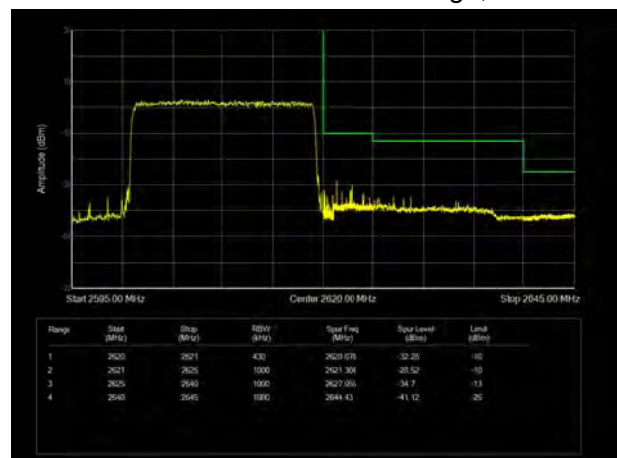
LTE Band 38 16QAM 5MHz CH-High, 1 RB
