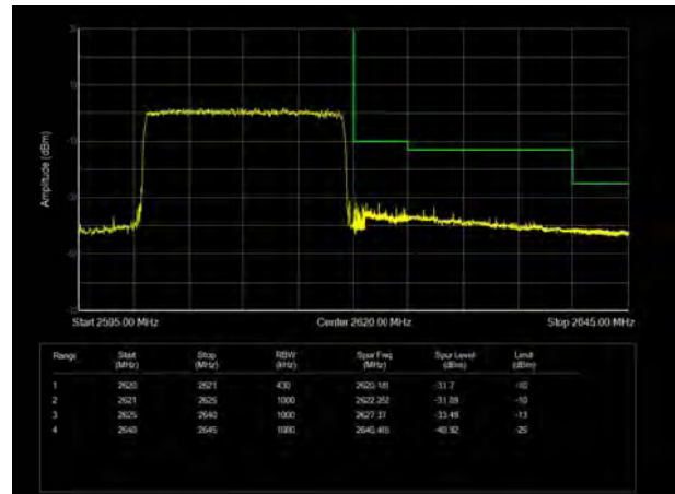
LTE Band 38 64QAM 5MHz CH-High, 1 RB
