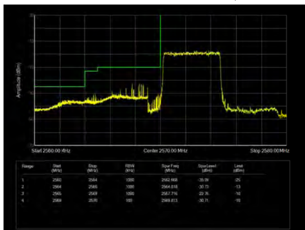
LTE Band 38 QPSK 10MHz CH-Low, 1 RB
