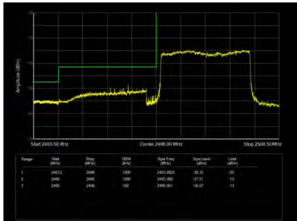
LTE Band 41 QPSK 15MHz CH-Low, 1 RB
