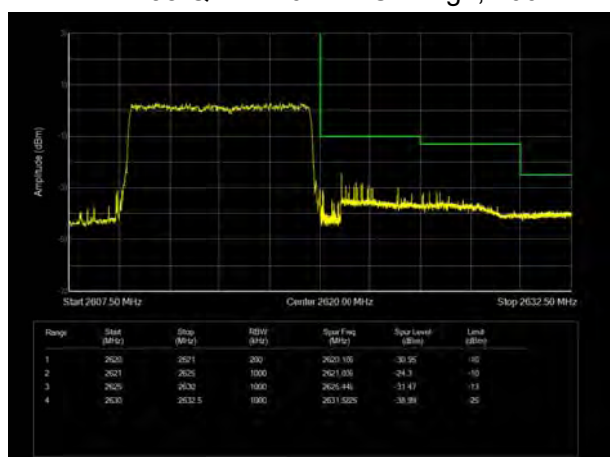
LTE Band 38 QPSK 15MHz CH-High, 1 RB
