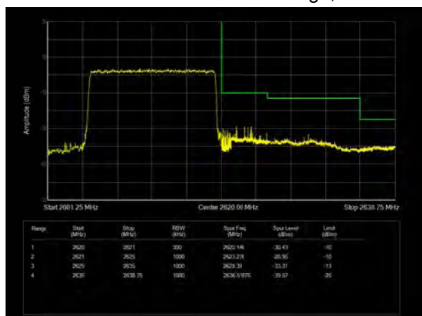
LTE Band 38 QPSK 15MHz CH-High, 100%RB
