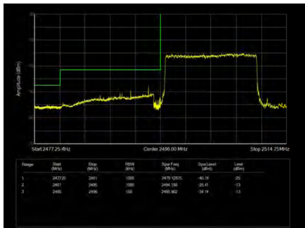
LTE Band 41 QPSK 15MHz CH-Low, 100%RB
