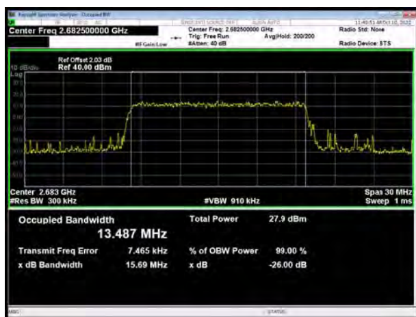
LTE Band 41 16QAM 15MHz CH-High
