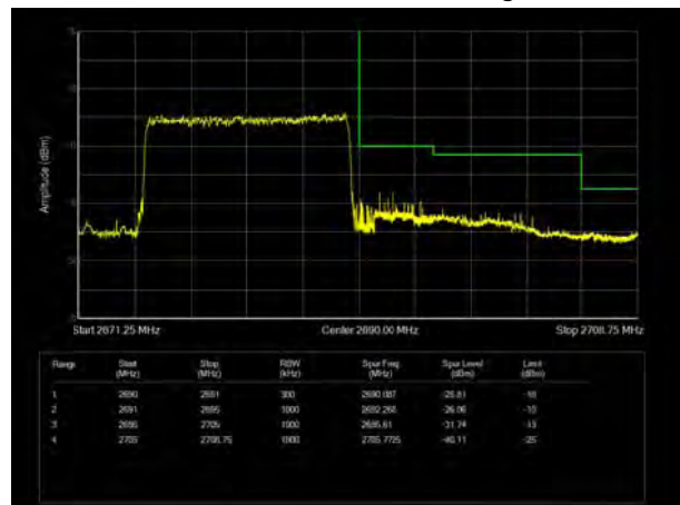
LTE Band 41 QPSK 15MHz CH-High, 100%RB
