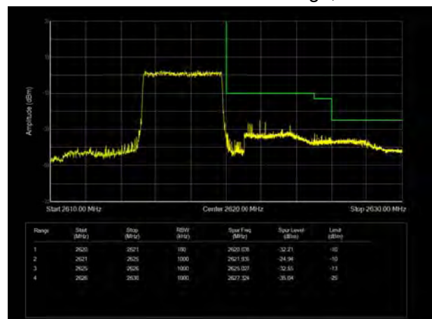
LTE Band 38 QPSK 10MHz CH-High, 1 RB
