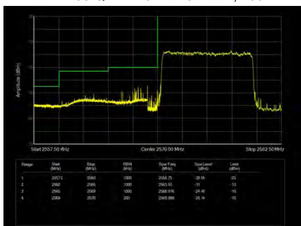
LTE Band 38 QPSK 15MHz CH-Low, 1 RB
