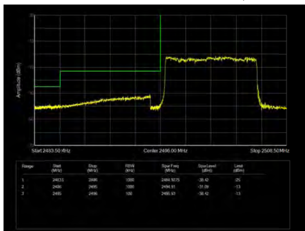
LTE Band 41 64QAM 15MHz CH-Low, 1 RB
