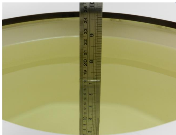
Fig 11.1 Photo of Liquid Height for Body SAR
