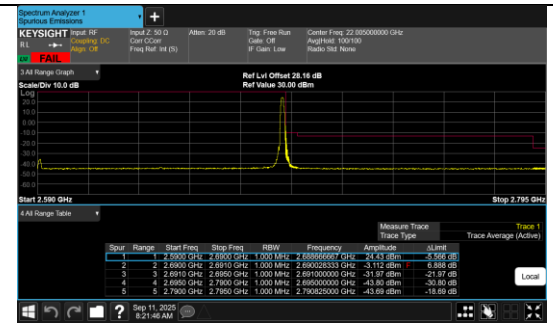
Conducted Band Edge Band 41 100MHz/2640.0/High BPSK 1@272
