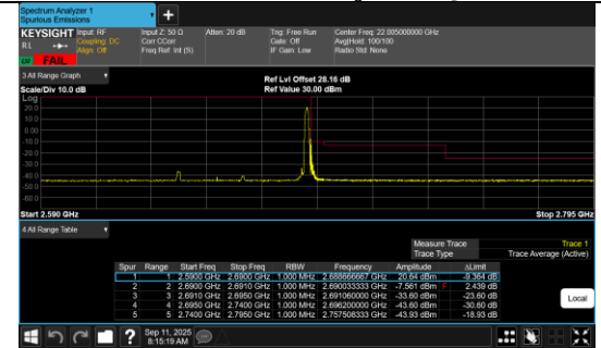
Conducted Band Edge Band 41 50MHz/2664.99/High QPSK 1@132
