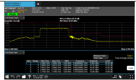
Conducted Band Edge Band 41 50MHz/2664.99/High BPSK 128@0
