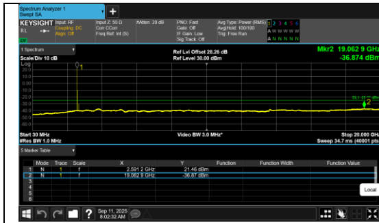
30.0MHz-20000MHz Band 41 100MHz/2640.0/High BPSK 1@0
