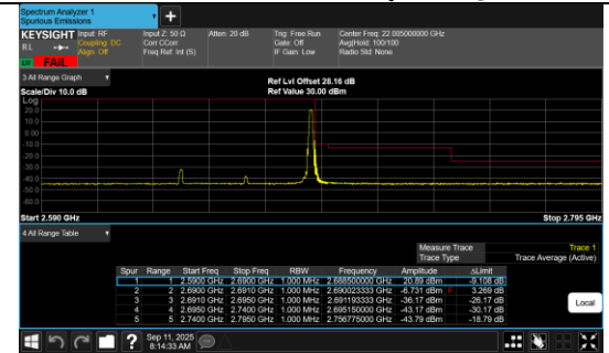
Conducted Band Edge Band 41 50MHz/2664.99/High BPSK 1@132
