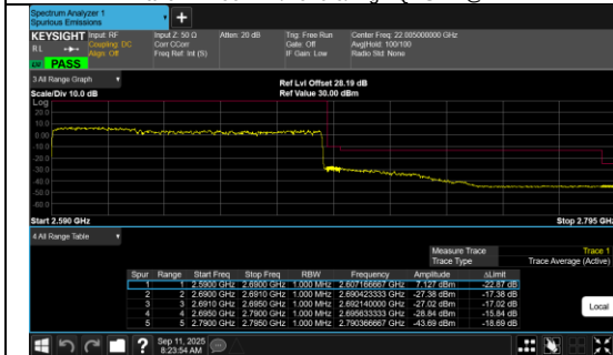
Conducted Band Edge Band 41 100MHz/2640.0/High QPSK 270@0
