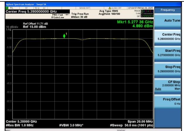
Mode:802.11n HT20 Frequency:5280MHz Ant:Chain0
