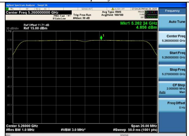
Mode:802.11n HT20 Frequency:5260MHz Ant:Chain1
