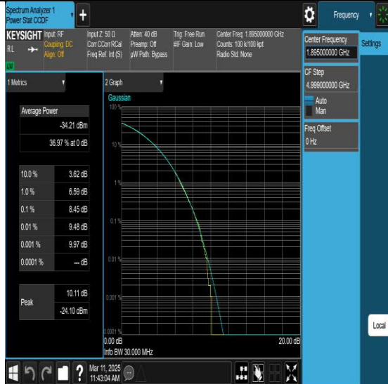
NTNV-N2-PC3-15-30-H-DFT-QPSK-Edge 1RB Left-PASS
