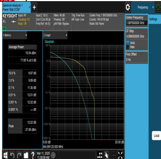
NTNV-N2-PC3-15-25-H-DFT-QPSK-Edge 1RB Left-PASS
