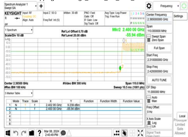
Hopping Band Edge_GFSK_1M_DH5_2480MHz
