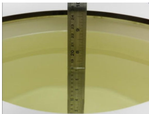
Fig 11.2 Photo of Liquid Height for Body SAR
