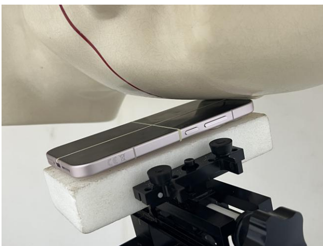
Left Tilted, Test Separation 0 mm
