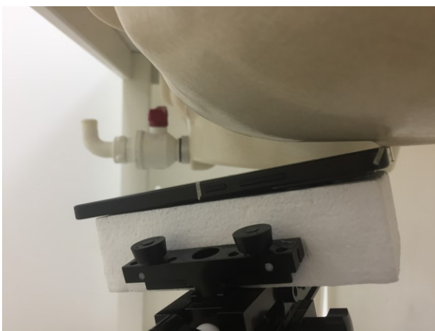
Left Tilted, Test Separation 0 mm
