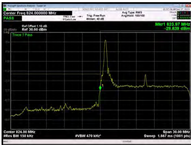
LTE Band 26 64QAM 15MHz CH-Low 100%RB
