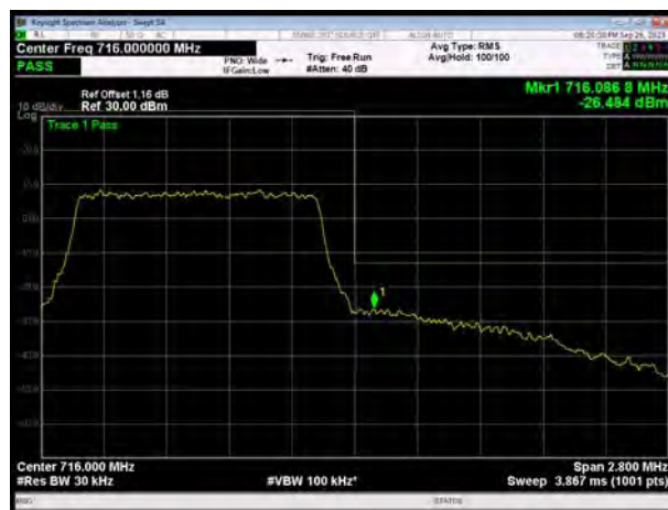
LTE Band 12 64QAM 1.4MHz CH-High, 100%RB
