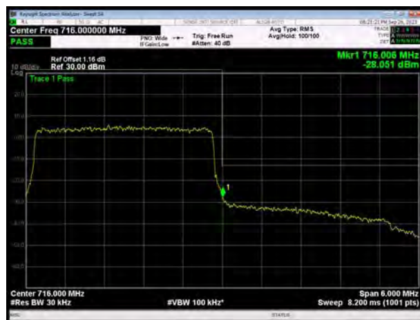
LTE Band 12 QPSK 5MHz CH-High, 1 RB
