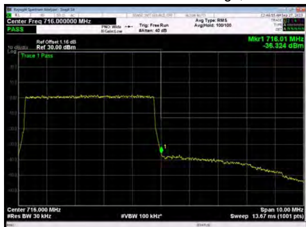
LTE Band 17 64QAM 10MHz CH-High, 1 RB
