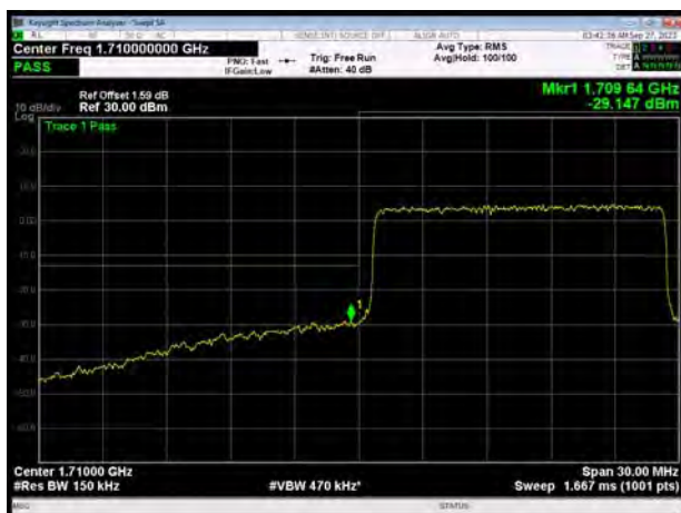
LTE Band 66 16QAM 20MHz CH-Low, 1 RB
