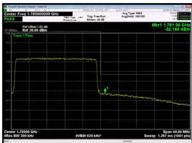
LTE Band 66 64QAM 20MHz CH-High, 100%RB
