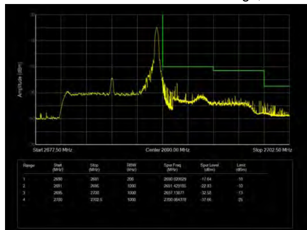
LTE Band 41 16QAM 10MHz CH-High, 100%RB
