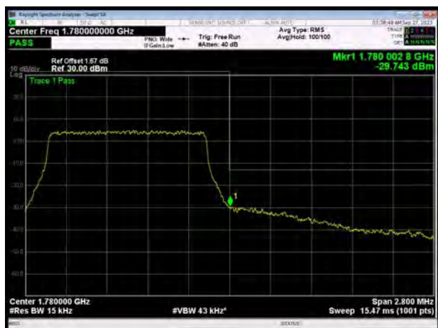
LTE Band 66 64QAM 3MHz CH-High, 1 RB
