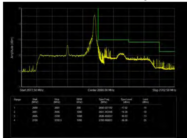
LTE Band 41 QPSK 10MHz CH-High, 1 RB
