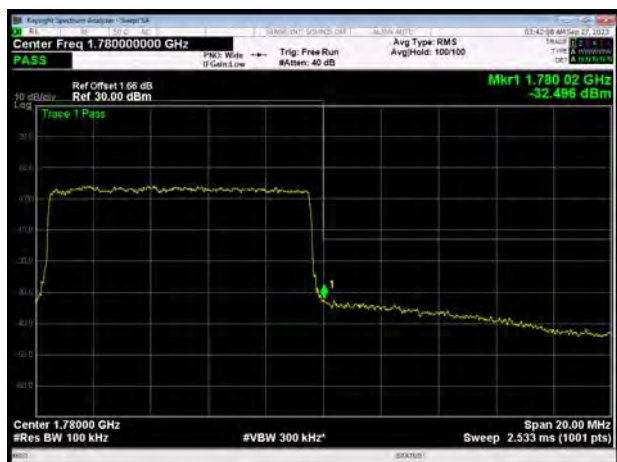
LTE Band 66 64QAM 15MHz CH-High, 1 RB
