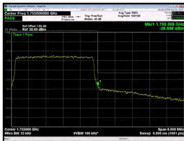
LTE Band 4 16QAM 5MHz CH-High, 1 RB
