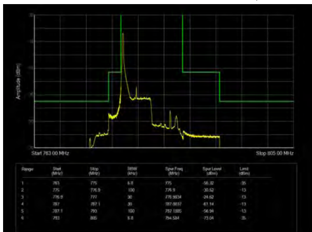
LTE Band 13 64QAM 5MHz CH-Low, 1 RB
