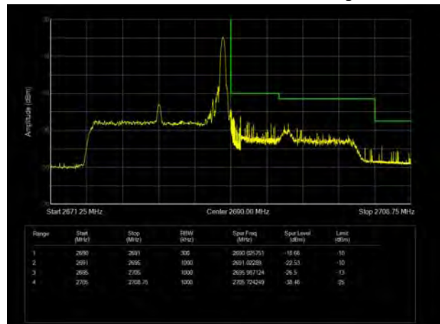
LTE Band 41 64QAM 15MHz CH-High, 1 RB
