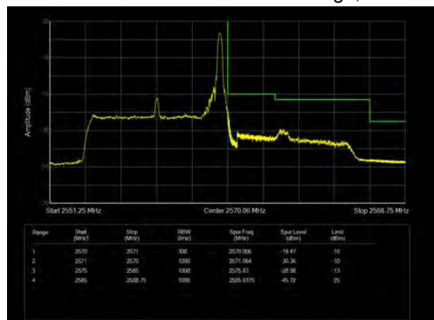
LTE Band 7 64QAM 15MHz CH-High, 1 RB
