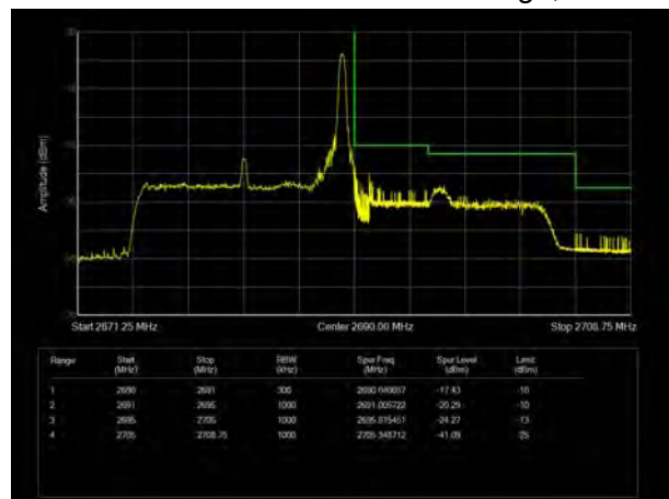
LTE Band 41 QPSK 15MHz CH-High, 100%RB
