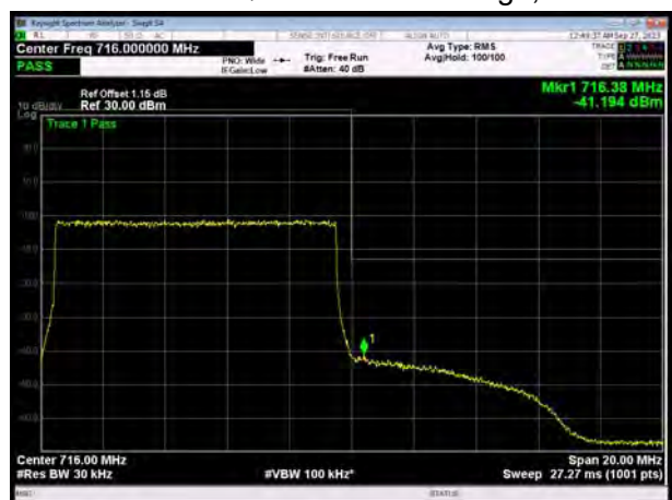
LTE Band 17 64QAM 5MHz CH-High, 1 RB
