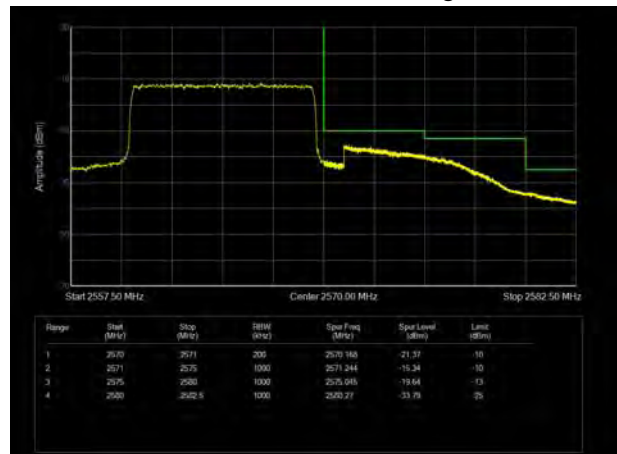
LTE Band 7 QPSK 15MHz CH-High, 1 RB
