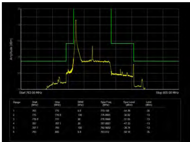
LTE Band 13 64QAM 10MHz CH-Low, 100%RB
