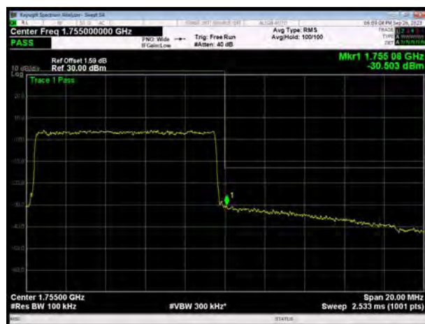
LTE Band 4 16QAM 15MHz CH-High, 1 RB
