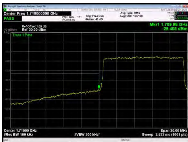
LTE Band 66 16QAM 15MHz CH-Low, 1 RB
