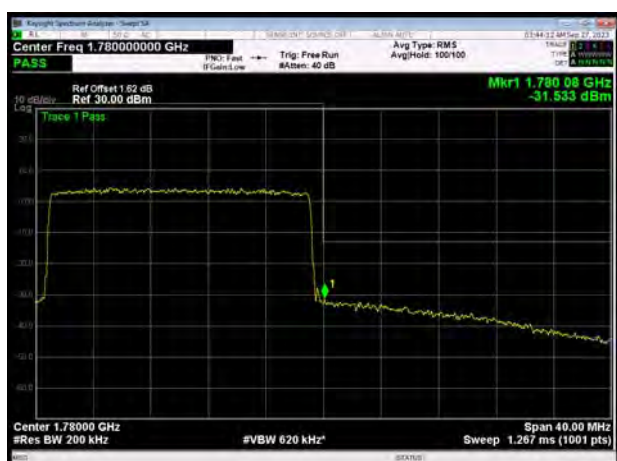
LTE Band 66 16QAM 20MHz CH-High, 100%RB
