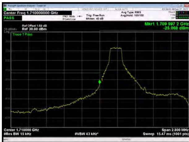
LTE Band 66 64QAM 1.4MHz CH-Low, 100%RB
