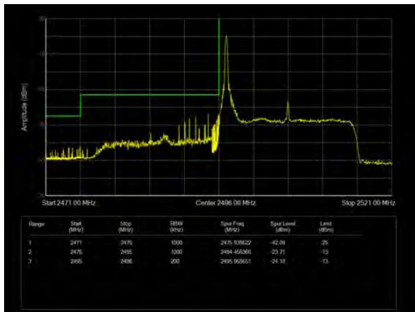
LTE Band 41 16QAM 20MHz CH-Low, RB 1
