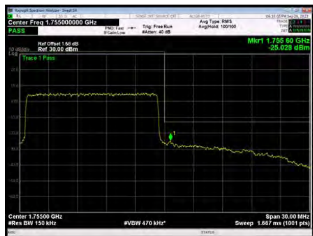
LTE Band 4 QPSK 20MHz CH-High, 1 RB
