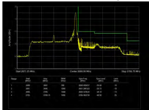
LTE Band 41 16QAM 15MHz CH-High, 100%RB
