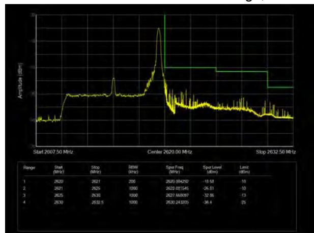
LTE Band 38 16QAM 10MHz CH-High, 100%RB
