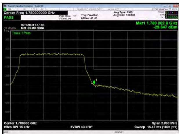
LTE Band 66 16QAM 3MHz CH-High, 1 RB
