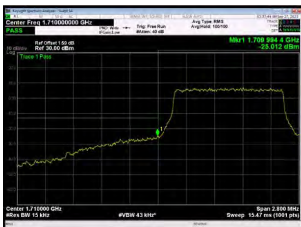
LTE Band 66 QPSK 3MHz CH-Low, 1 RB
