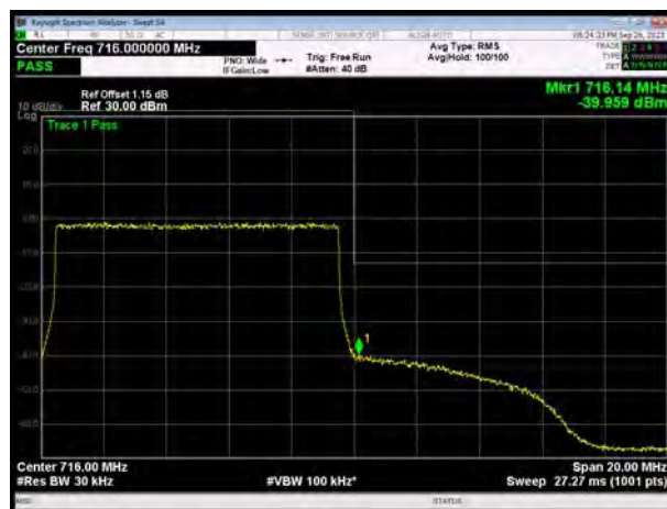
LTE Band 12 64QAM 1.4MHz CH-High, 1 RB
