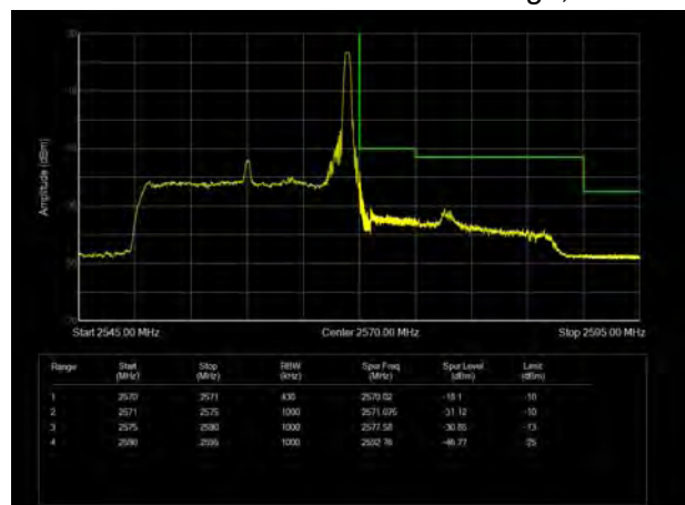
LTE Band 7 16QAM 20MHz CH-High, 1 RB
