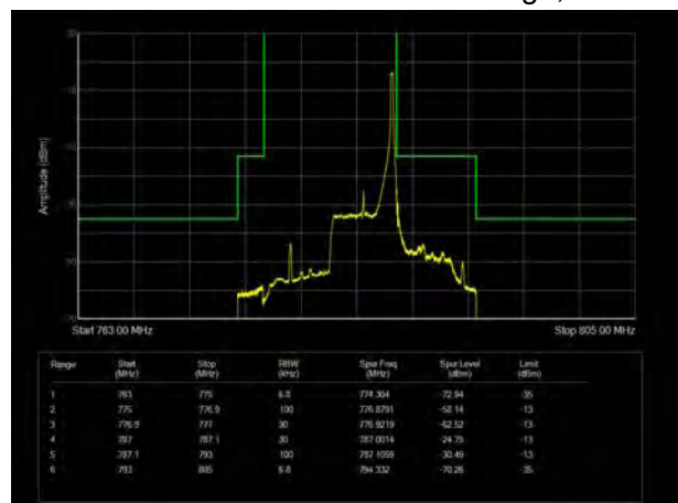
LTE Band 13 16QAM 5MHz CH-High, 100%RB
