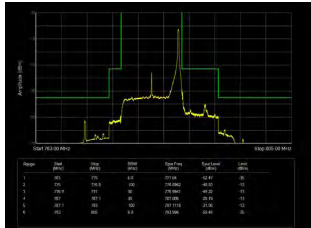
LTE Band 13 QPSK 10MHz CH-High, 1 RB
