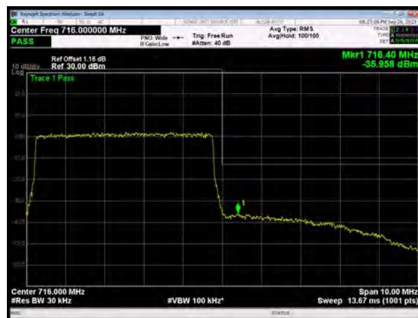
LTE Band 12 64QAM 10MHz CH-High, 1 RB
