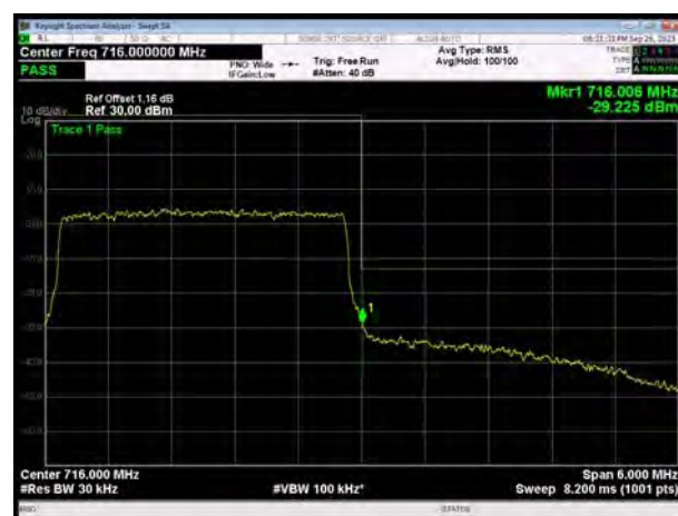
LTE Band 12 16QAM 3MHz CH-High, 100%RB
