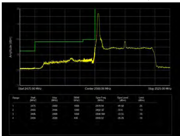
LTE Band 7 64QAM 20MHz CH-Low, 100%RB
