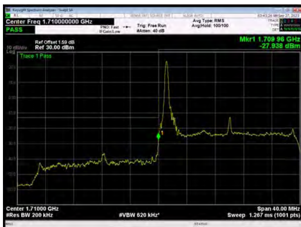
LTE Band 66 QPSK 20MHz CH-Low, 100%RB
