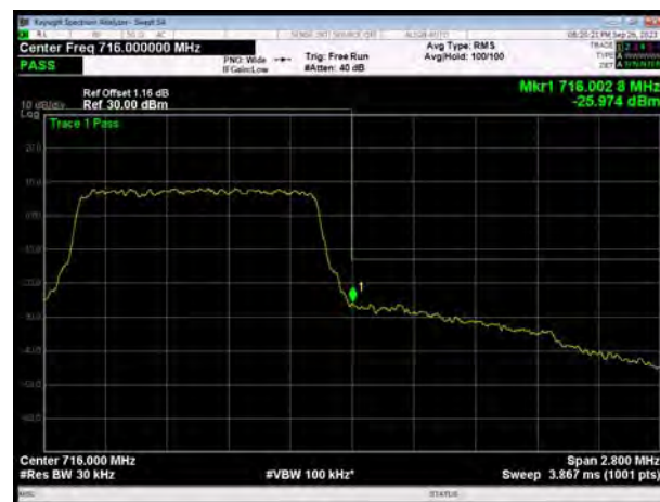
LTE Band 12 16QAM 3MHz CH-High, 1 RB
