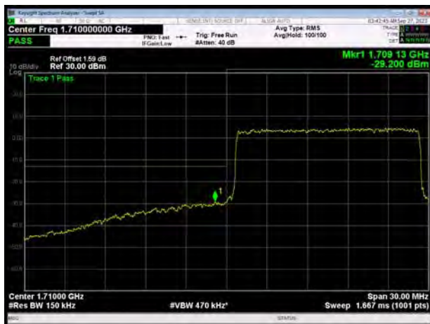
LTE Band 66 64QAM 20MHz CH-Low, 1 RB
