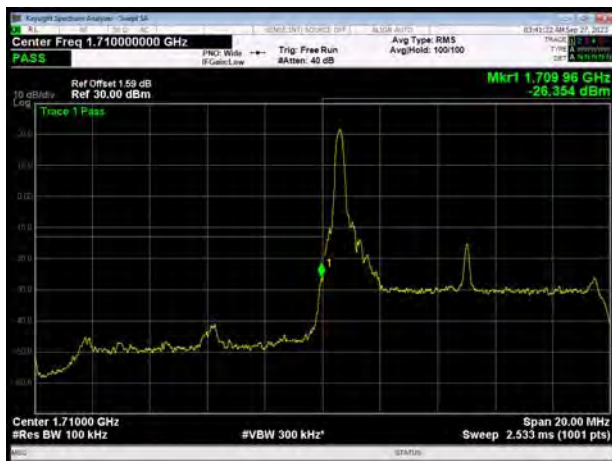
LTE Band 66 16QAM 10MHz CH-Low, 100%RB
