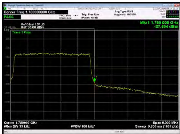
LTE Band 66 16QAM 5MHz CH-High, 1 RB
