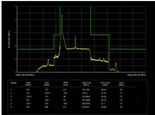
LTE Band 13 QPSK 10MHz CH-Low, 1 RB
