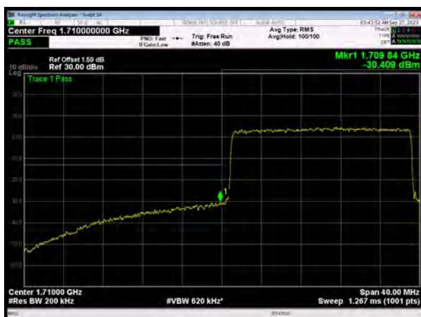
LTE Band 66 64QAM 20MHz CH-Low, 100%RB
