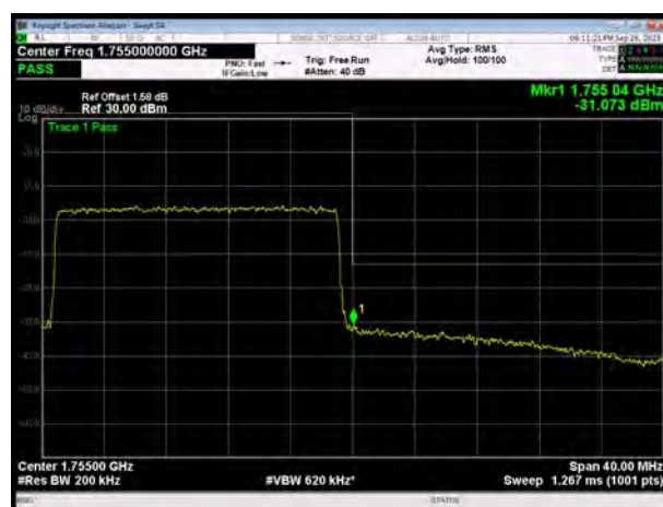
LTE Band 4 16QAM 20MHz CH-High, 100%RB
