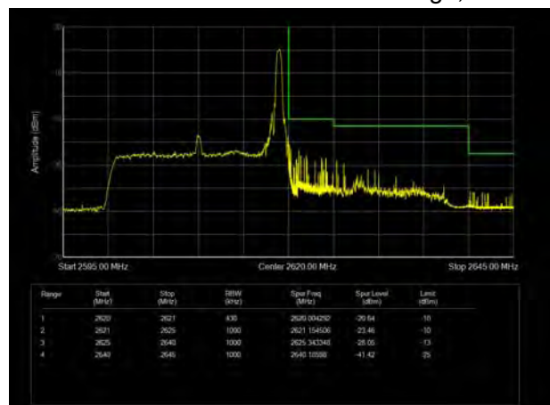
LTE Band 38 16QAM 20MHz CH-High, 1 RB
