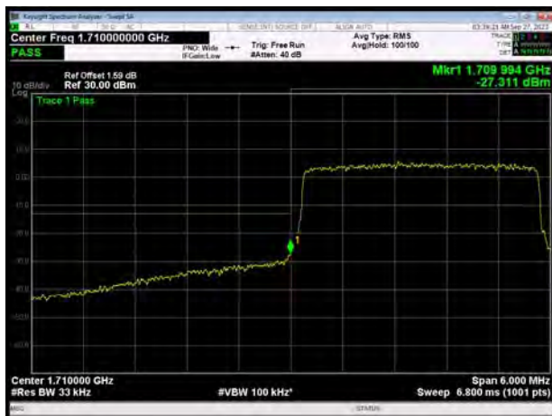
LTE Band 66 64QAM 5MHz CH-Low, 1 RB
