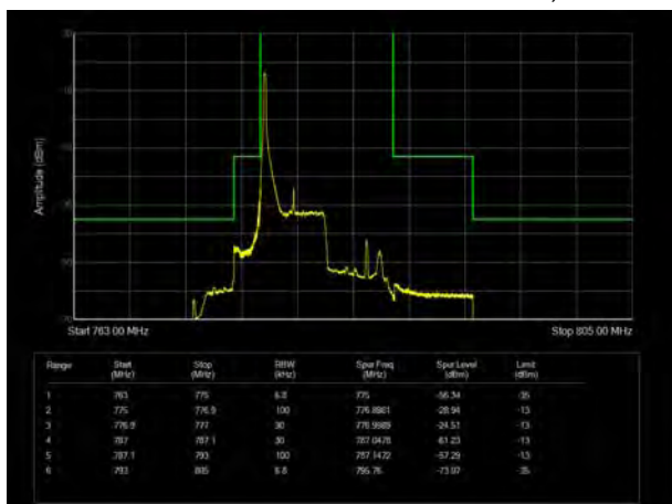
LTE Band 13 16QAM 5MHz CH-Low, 100%RB
