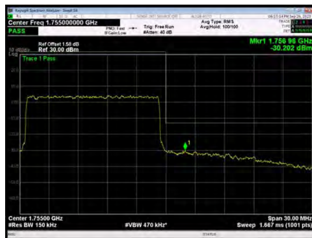
LTE Band 4 16QAM 20MHz CH-High, 1 RB
