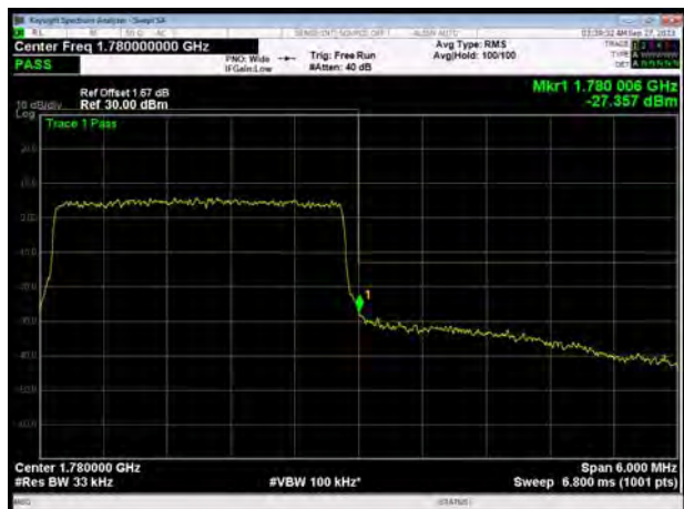
LTE Band 66 QPSK 5MHz CH-High, 1 RB
