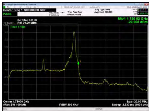
LTE Band 66 64QAM 10MHz CH-High, 100%RB
