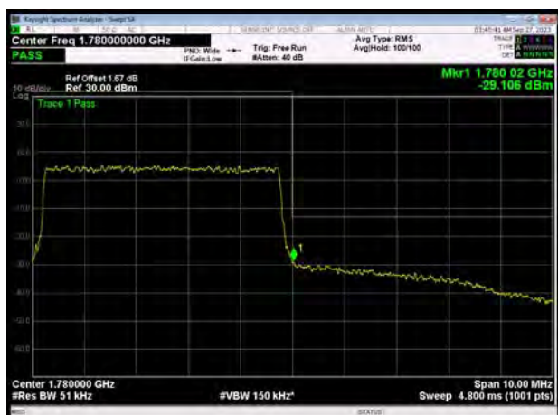
LTE Band 66 QPSK 5MHz CH-High, 100%RB
