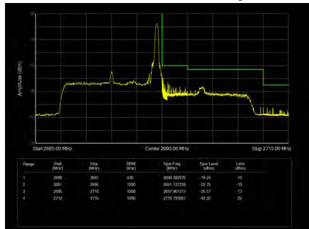
LTE Band 41 QPSK 20MHz CH-High, 100%RB
