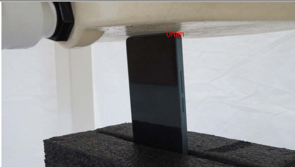
Picture 17: Top Edge, the distance from EUT to the bottom of the Phantom is 0mm
