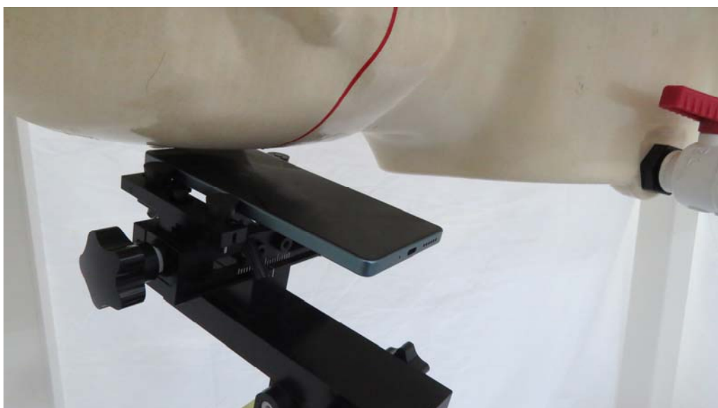
Picture 4: Right Hand Tilt 15 Degree Position
