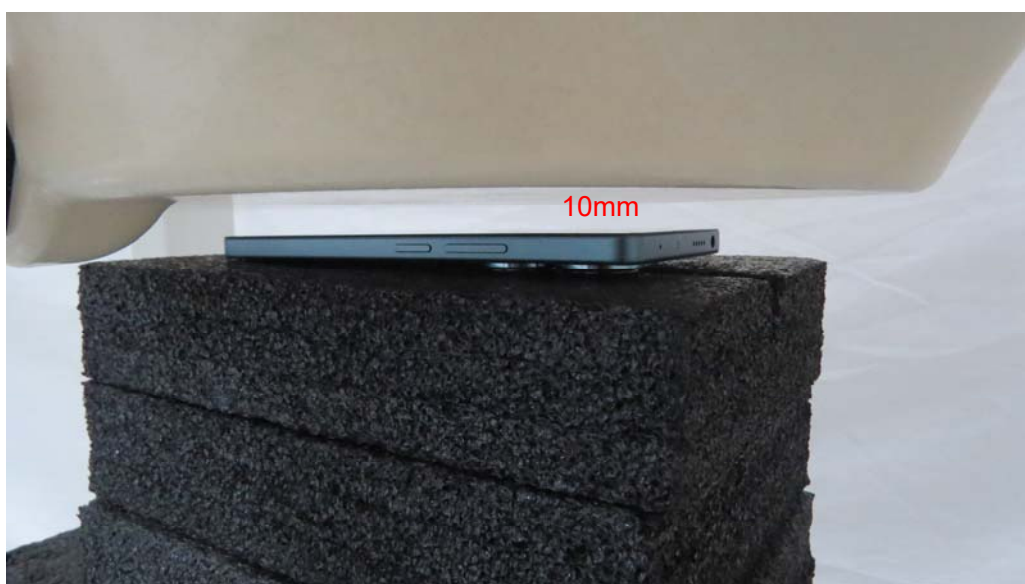
Picture 8: Front Side, the distance from EUT to the bottom of the Phantom is 10mm
