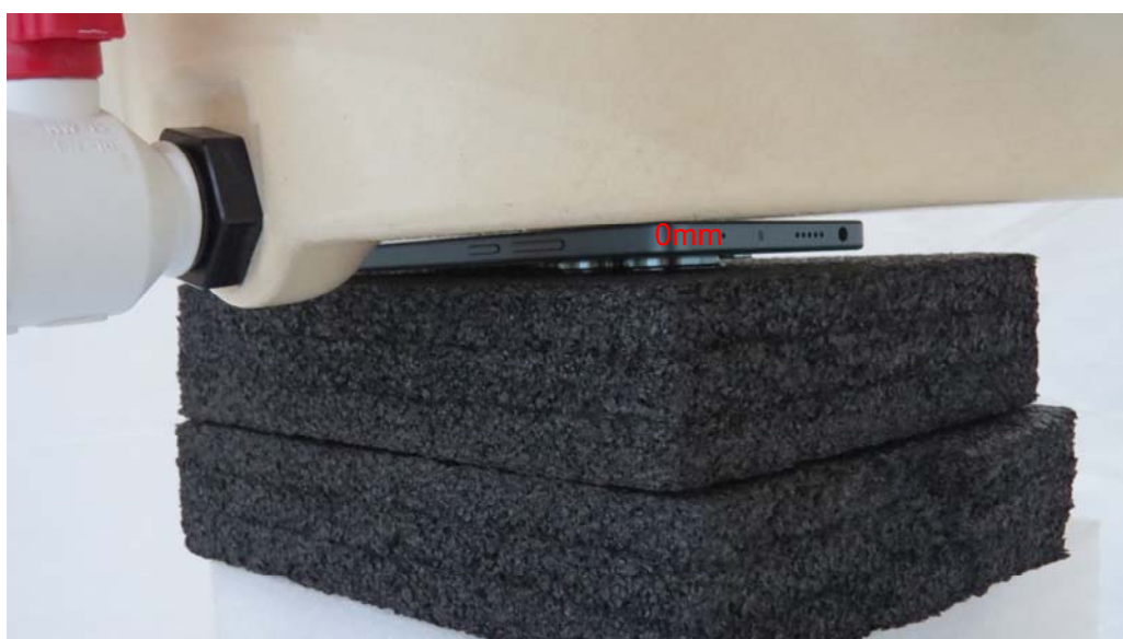
Picture 14: Front Side, the distance from EUT to the bottom of the Phantom is 0mm
