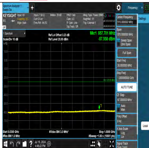
Band41 10MHz QPSK 40620 1RB#0 30~1000 30~1000
