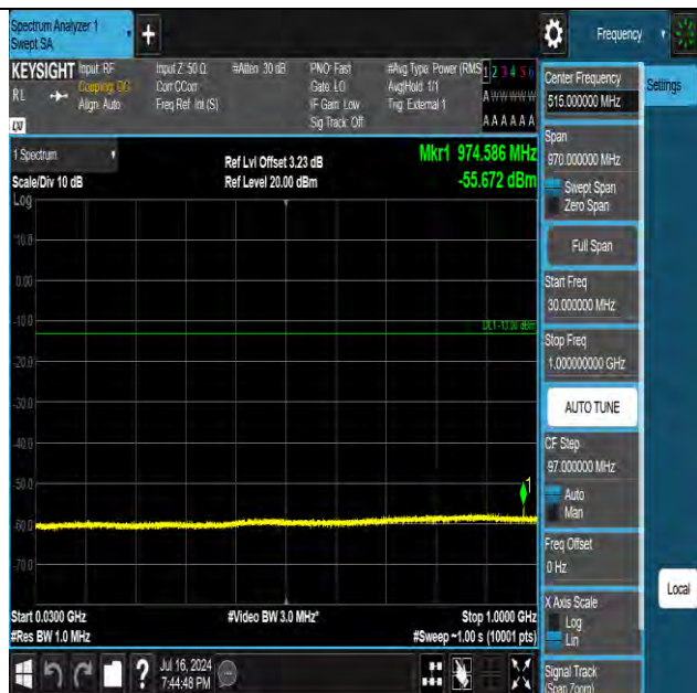
Band42 15MHz QPSK 43015 1RB#0 30~1000 30~1000
