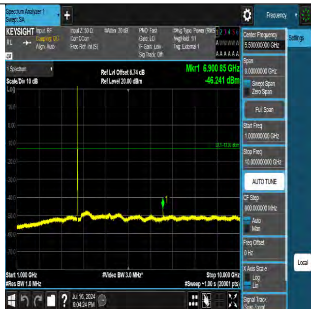
Band42 10MHz QPSK 42140 1RB#0 1000~10000 1000~10000
