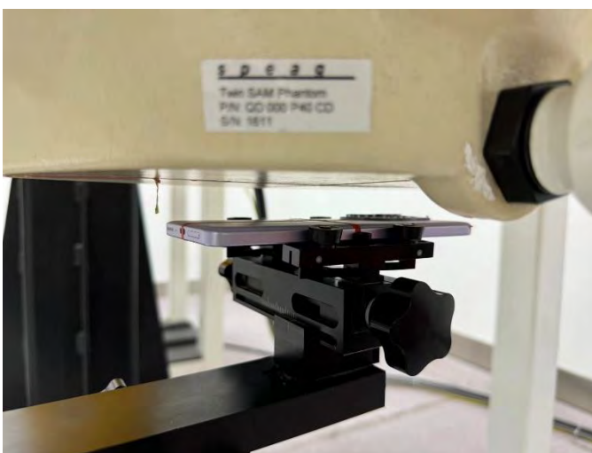
Rear Face of EUT with 2.0 cm Gap (Body-Worn Mode)
