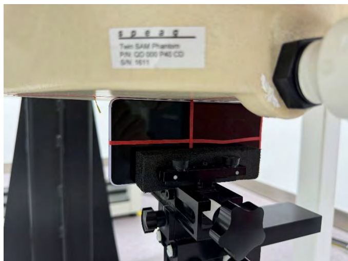
Left Side of EUT with 0 cm Gap (Limbs Mode)
