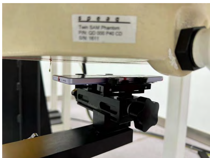
Front Face of EUT with 2.0 cm Gap (Body-Worn Mode)
