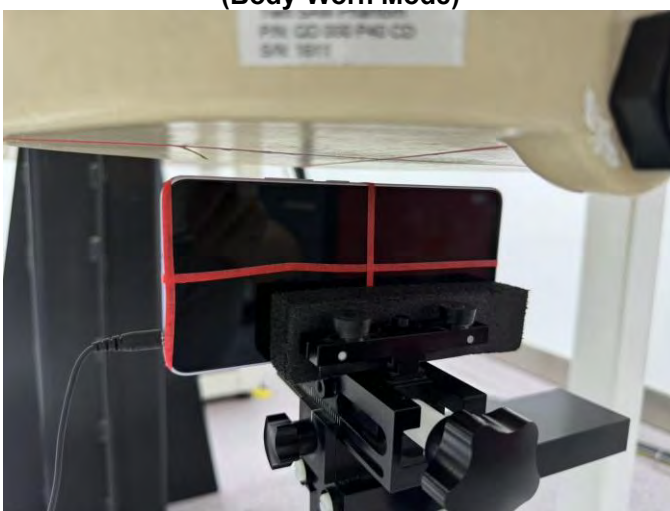
Right Side of EUT with 1 cm Gap (Body-Worn Mode)
