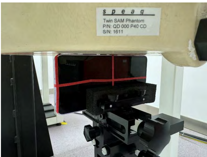
Right Side of EUT with 0 cm Gap (Limbs Mode)
