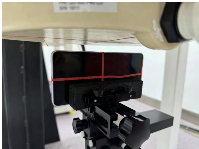
Left Side of EUT with 1.5 cm Gap (Body-Worn Mode)
