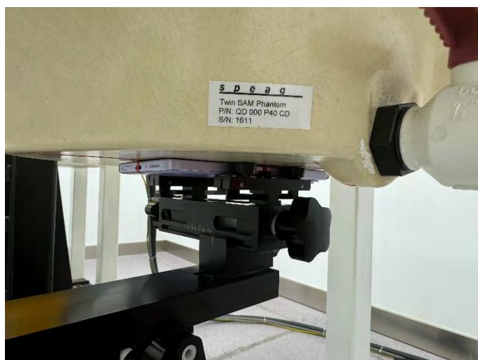
Front Face of EUT with 0 cm Gap (Limbs Mode)
