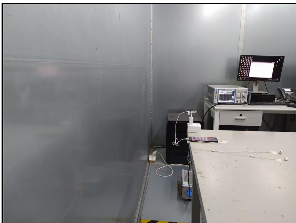
Fig. 4 Power line conducted emission setup photo
