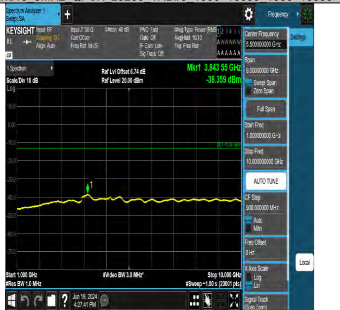
Band13 5MHz QPSK 23255 1RB#0 1000~10000 1000~10000
