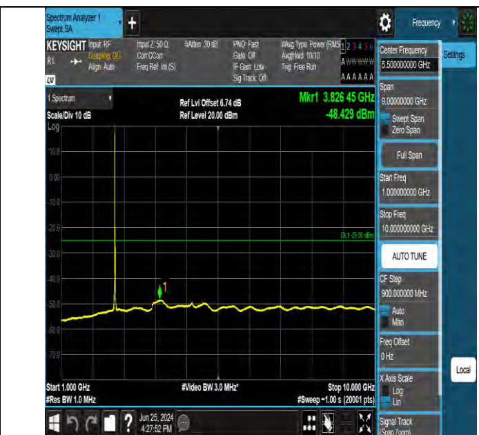
Band7 15MHz QPSK 21100 1RB#0 1000~10000 1000~10000
