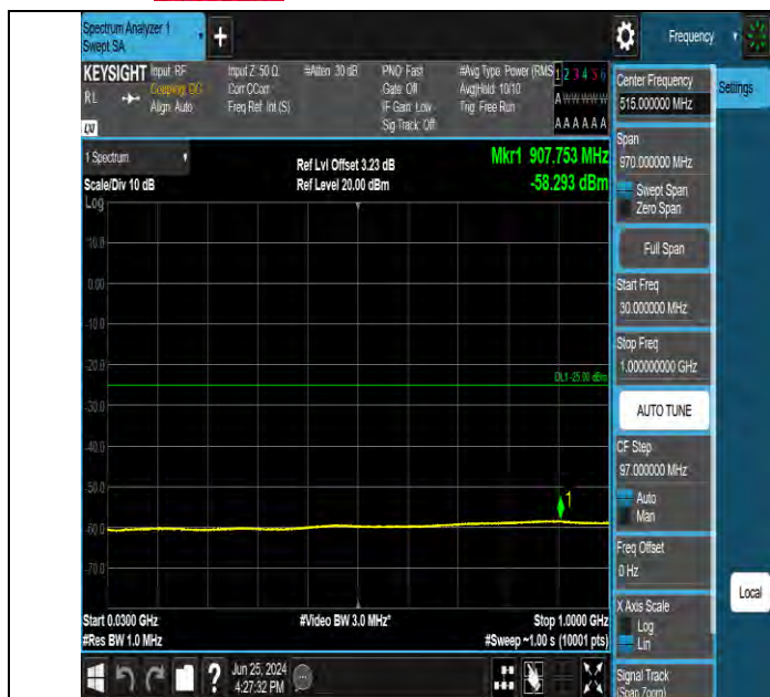
Band7 15MHz QPSK 21100 1RB#0 30~1000 30~1000
