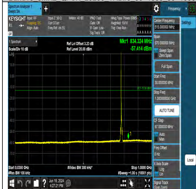
Band13 5MHz QPSK 23255 1RB#0 30~1000 30~1000
