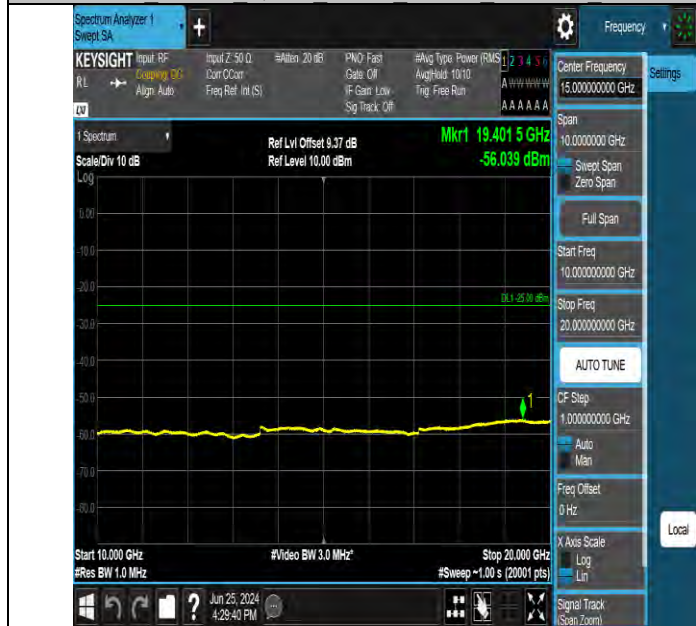
Band7 15MHz QPSK 21375 1RB#0 10000~20000 10000~20000
