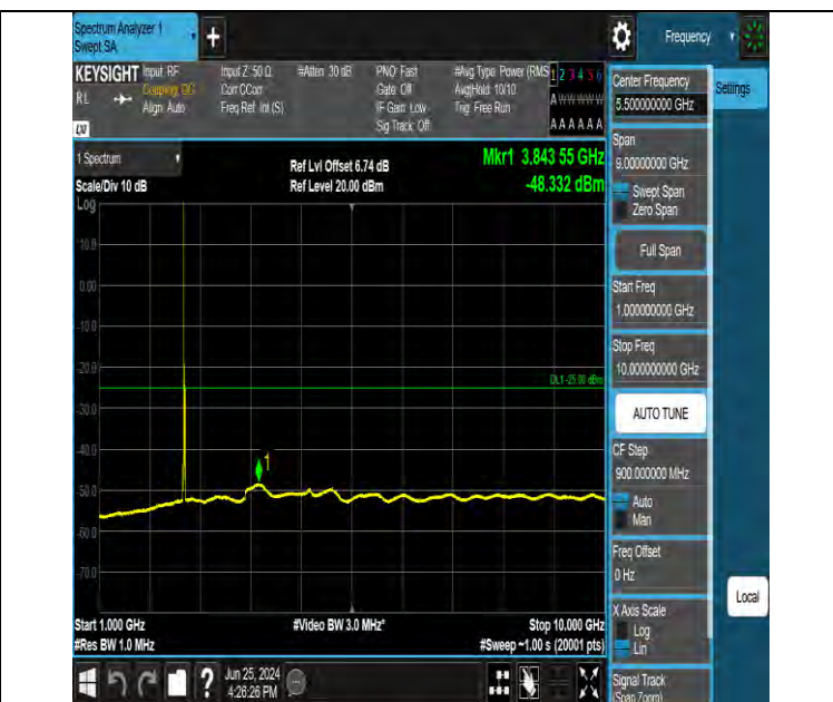
Band7 15MHz QPSK 20825 1RB#0 1000~10000 1000~10000
