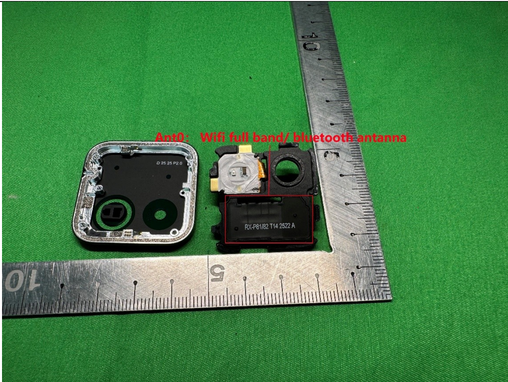
(18) EUT Photo Ant0: Wifi full band/Bluetooth antenna
