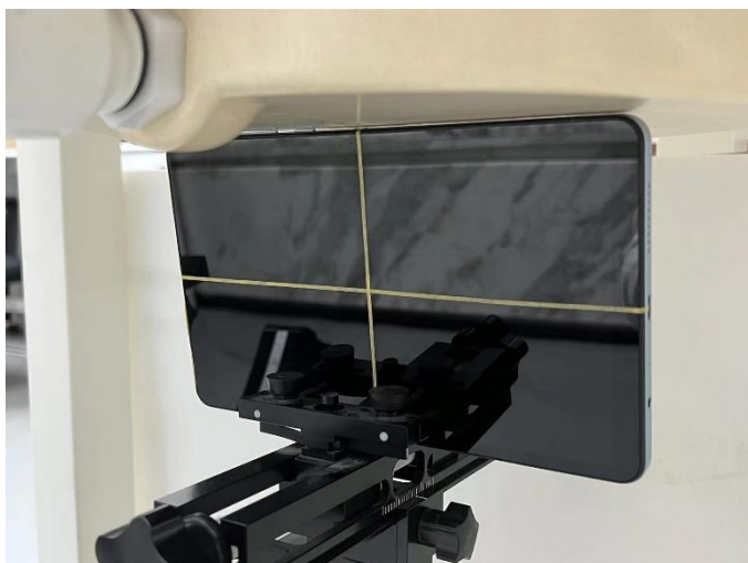
Right Side of EUT with 1 cm Gap (Body Mode)
