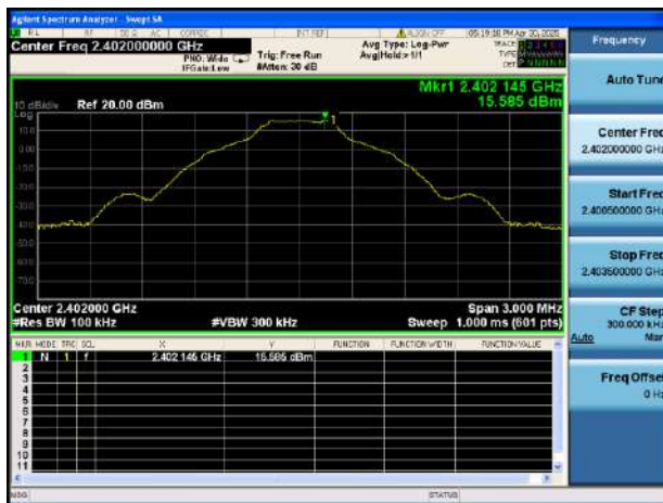
GFSK LOW CHANNEL, CARRIER LEVEL
