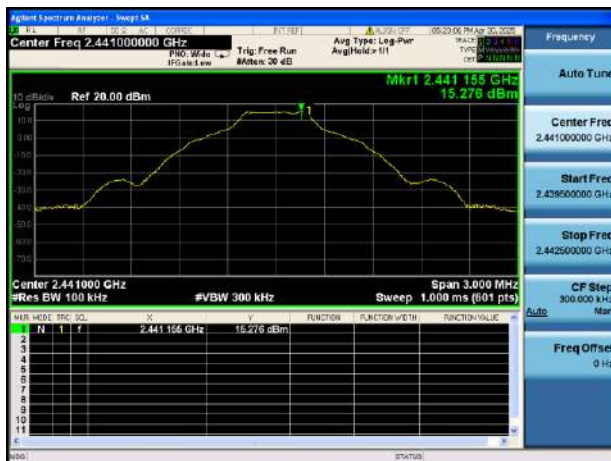
GFSK MIDDLE CHANNEL, CARRIER LEVEL
