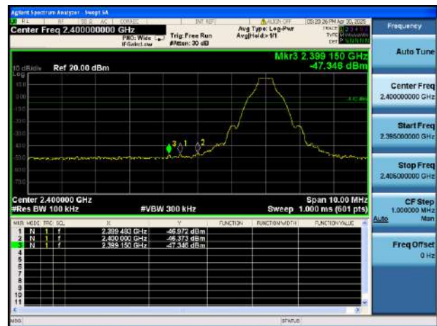
GFSK LOW CHANNEL, BAND EDGE
