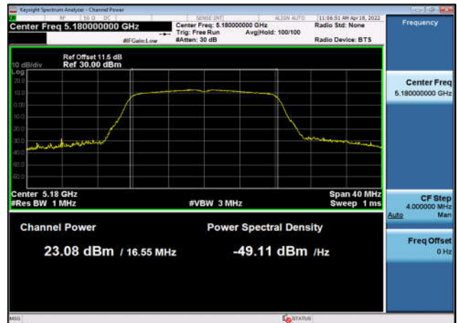
U-NII-1 Output Power-802.11a(20MHz) ,5240MHz,Ant1
