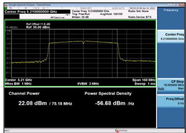
U-NII-1 Output Power-802.11ax(80MHz) ,5210MHz,Ant2
