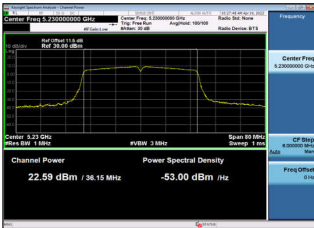
U-NII-1 Output Power-802.11ax(20MHz) ,5180MHz,Ant4
