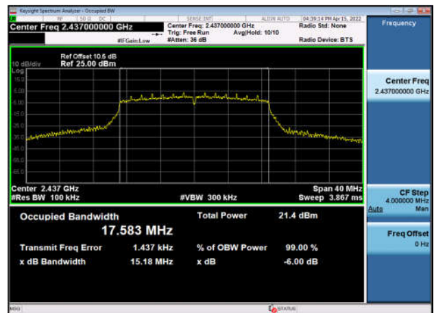
6dB Bandwidth-802.11ax(HE40),2422MHz ,Ant0
