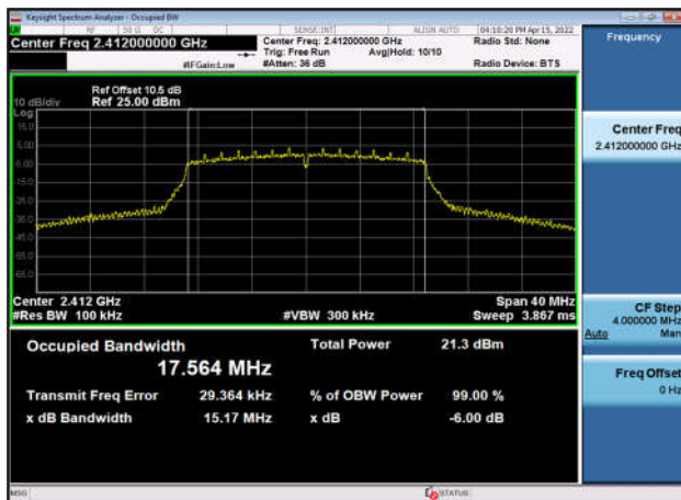
6dB Bandwidth-802.11ax(HE20),2462MHz ,Ant1
