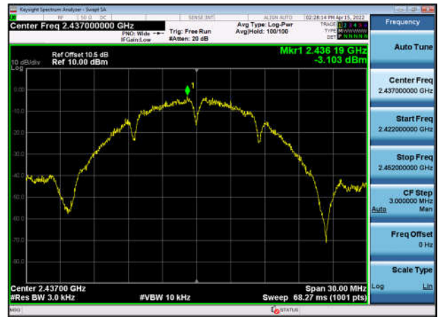
Power spectral density-802.11g ,2412MHz,Ant1
