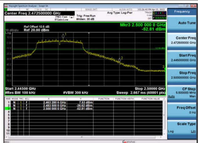
,Plot 2,Band Edge-802.11g,2462MHz ,Ant0
