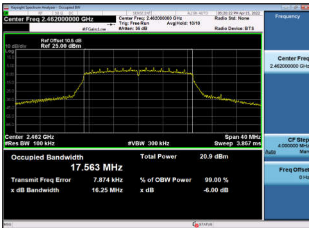
6dB Bandwidth-802.11n(HT40),2437MHz ,Ant1
