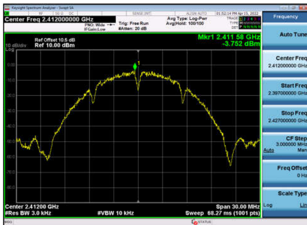
Power spectral density-802.11b ,2462MHz,Ant0
