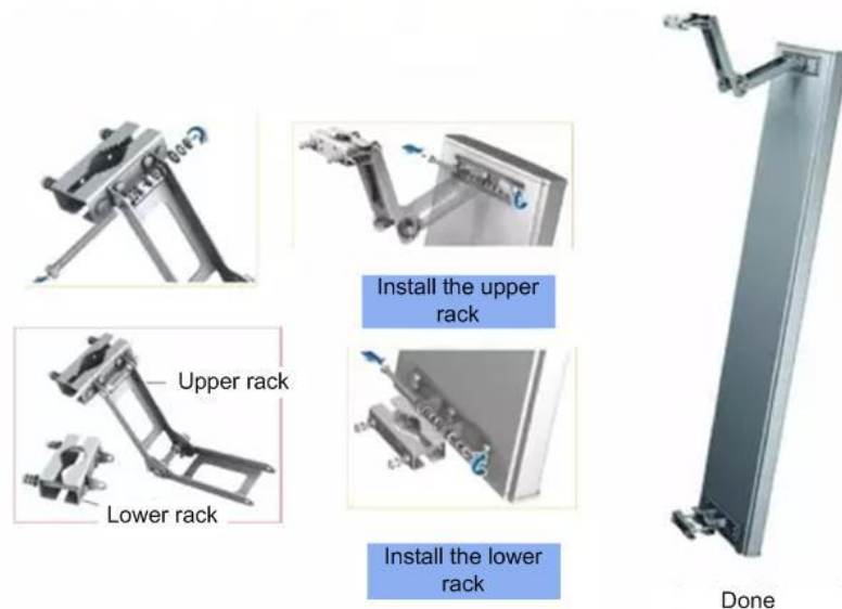
Figure 4-24 Assembling Procedure of Directional Antennas
