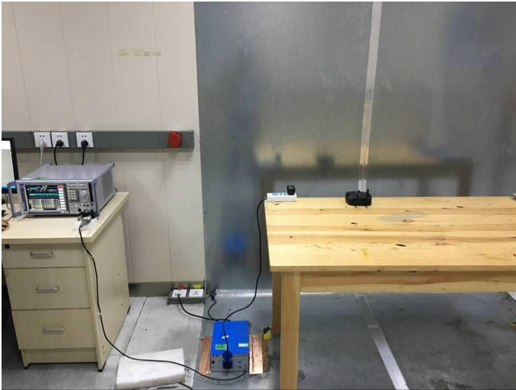
FCC RADIATED EMISSION TEST SETUP BELOW 1GHZ
