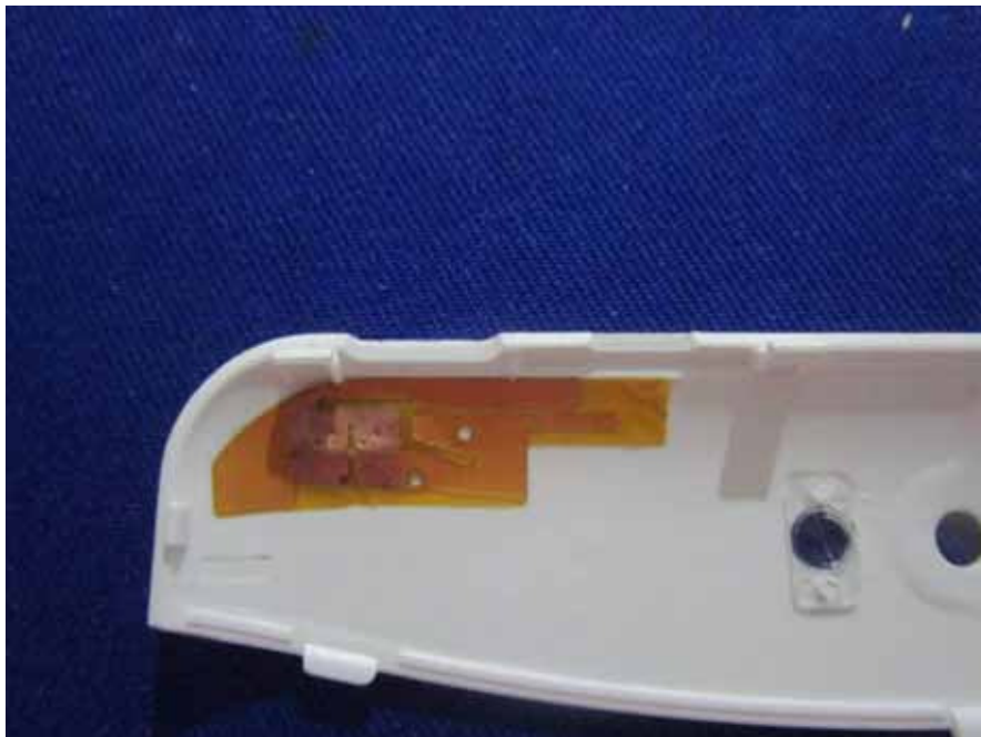
EUT –BT & Wifi Antenna View
