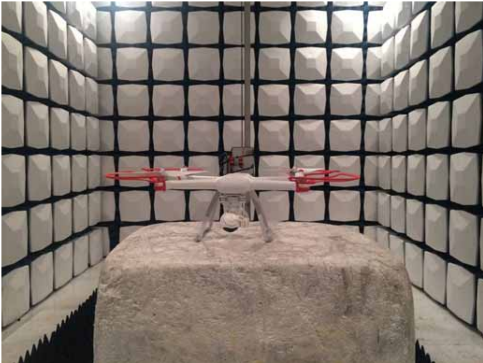
Description: Radiated Emission Test Setup for 1~18GHz
