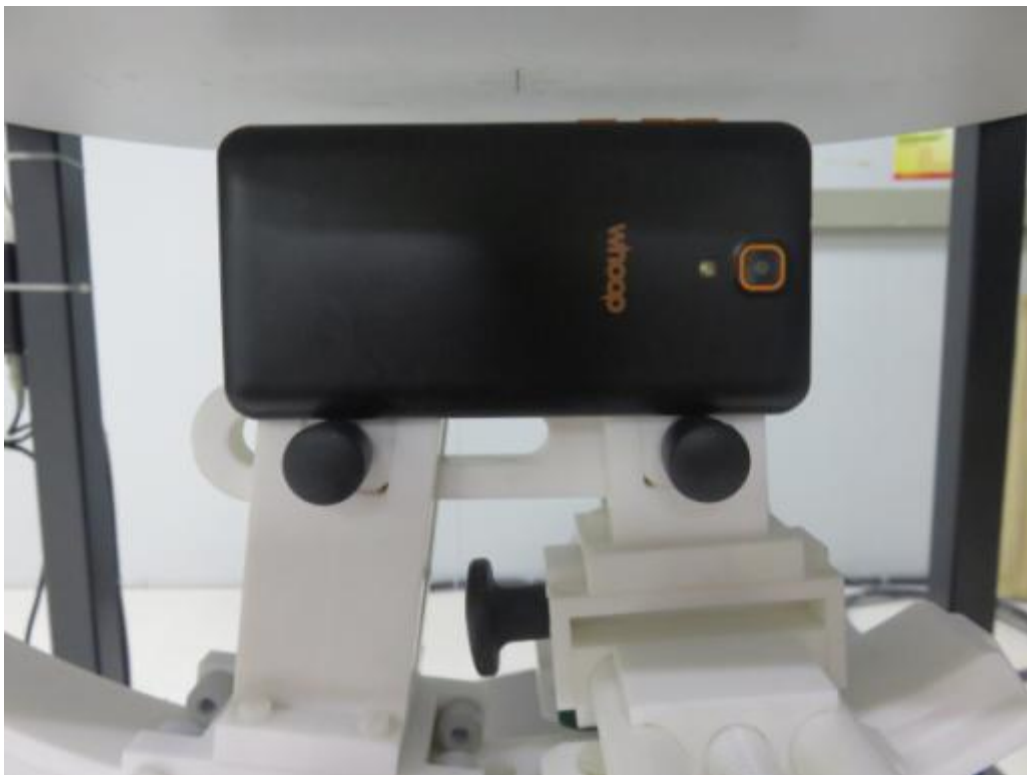
10mm body-worn Left Side Setup Photo(hotspot)
