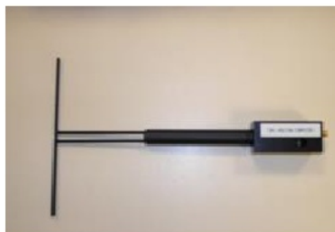
Figure 1 – Satimo COMOSAR Validation Dipole
