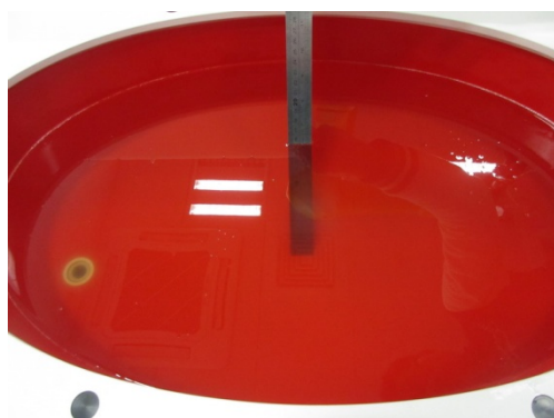
Liquid depth in the flat Phantom ( \geq 15\text{cm} depth) HSL(750MHz)
