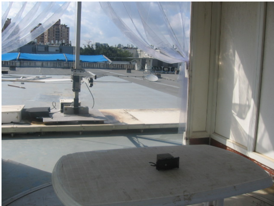
Radiated Emission Test, 200-1000MHz
