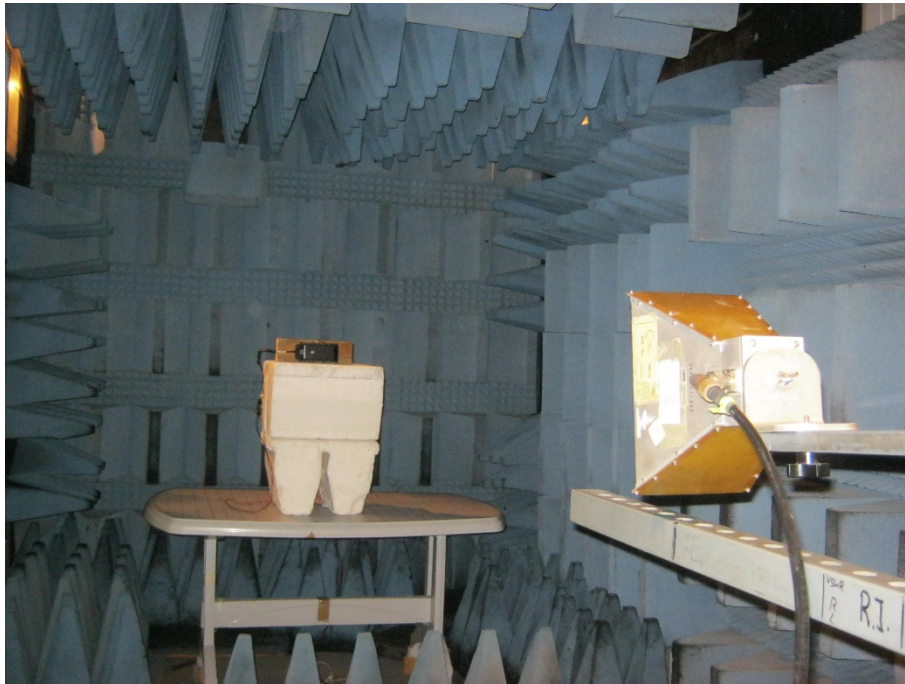
Radiated Emission Test, 1-18GHz
