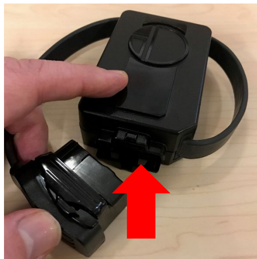
Fasten OBDII connector to enclosure
