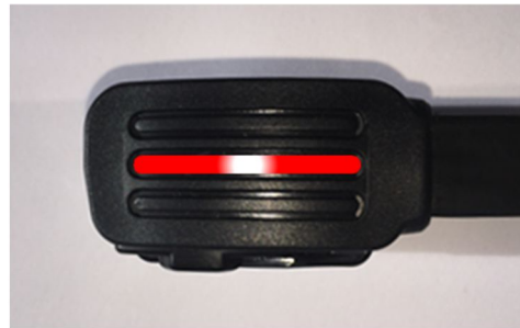
Figure 10 Solid Red LED Indicates Failed In-Fleet
