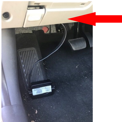
UTP 1.0 plugged into OBD-II port
