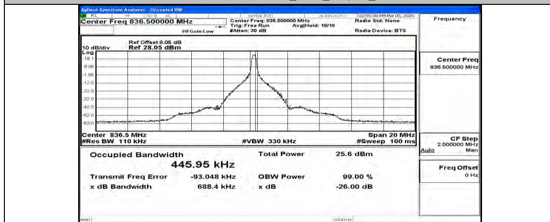
Channel Bandwidth: 10 MHz_MCH_16QAM_1RB#49
