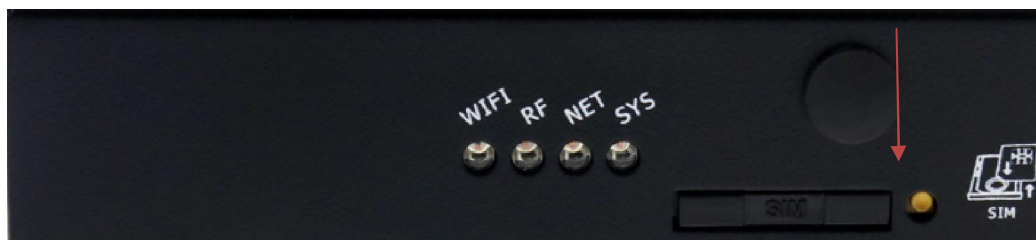
Figure 3-1 Pop out SIM slot
