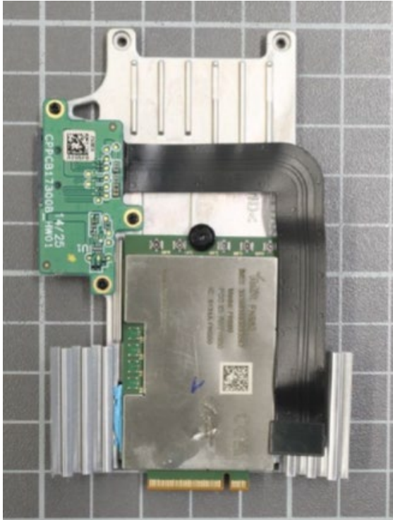
5G – MODULE – TOP View
