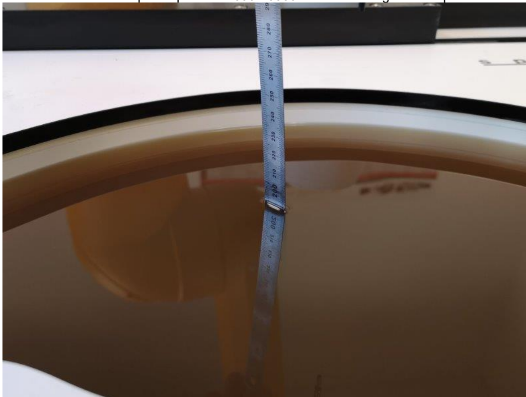
Photo 1: Liquid depth HBBL600-10000MHz Simulating Head Liquid
