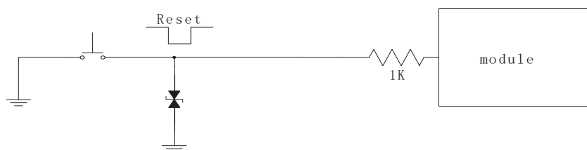
Figure 4.7: Reference design of key reset circuit
