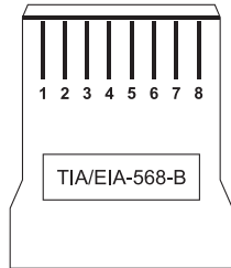
Figure 4. EIA/TIA 568B Termination Pattern
