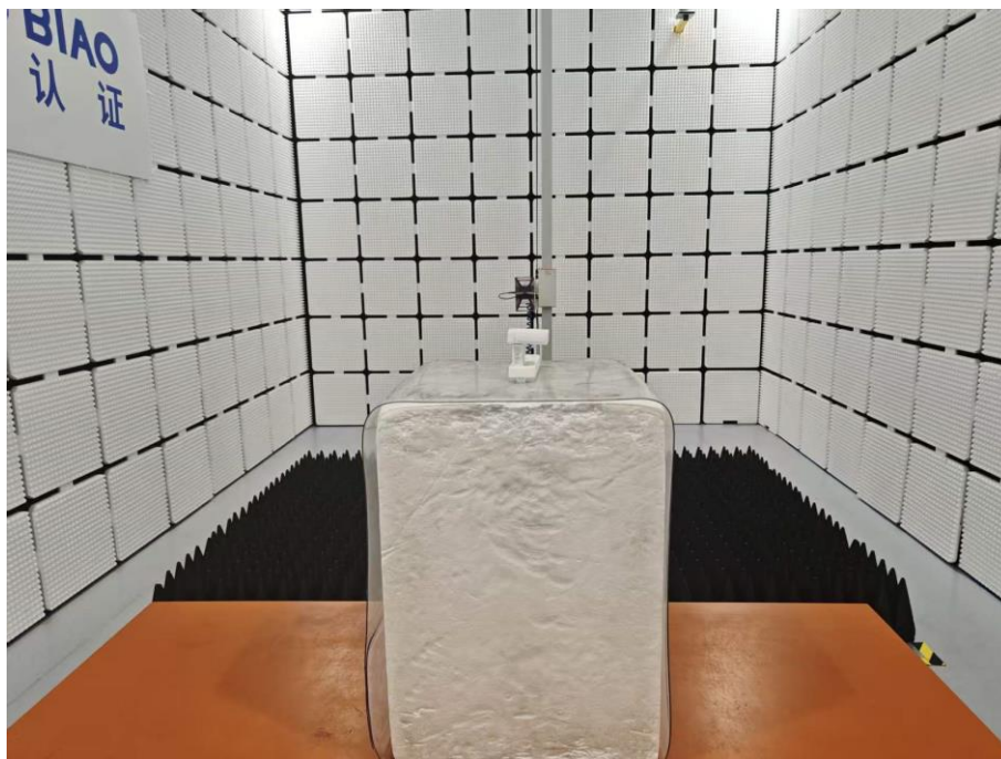
Radiated Emission Above 1GHz
