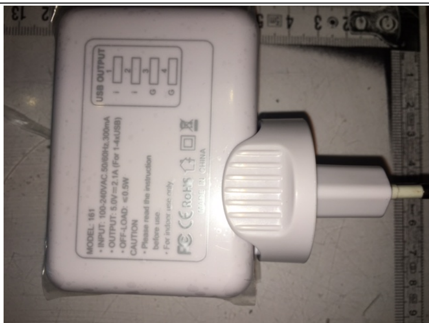
Power supply marking plate
