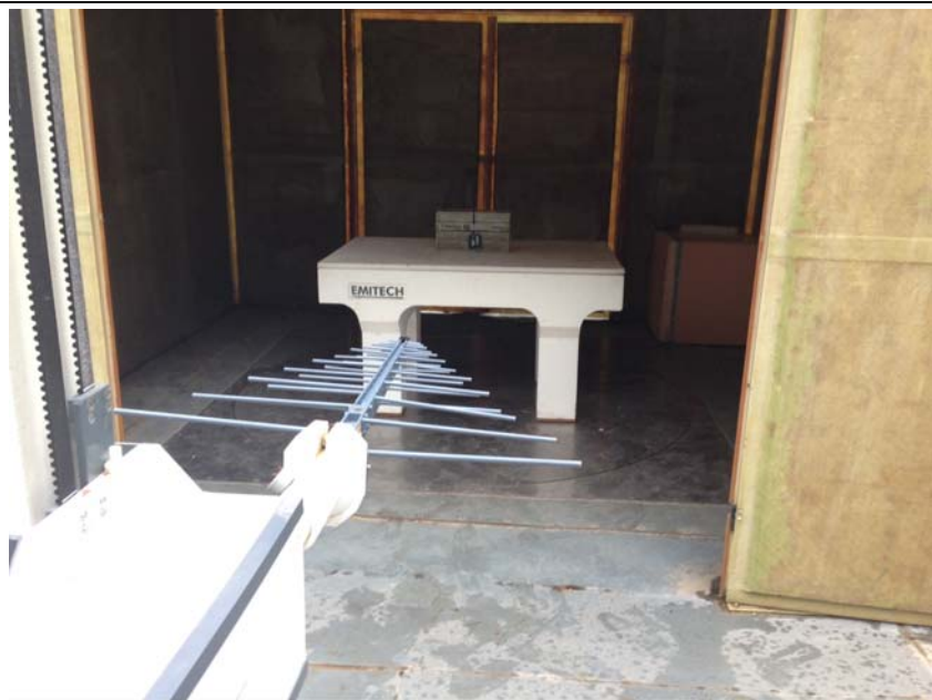
Open area test site measurements
