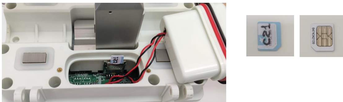
Figure 3: Inserting micro-SIM card into SIM socket
