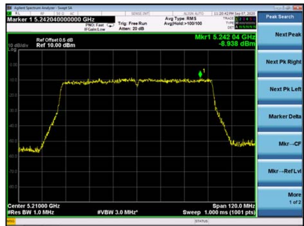
(802.11ac80) PSD plot on channel 42
