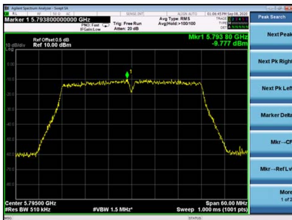
(802.11n40) PSD plot on channel 159
