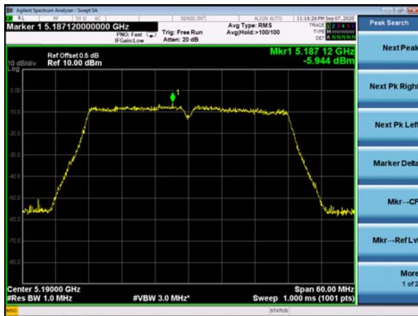
(802.11ac40) PSD plot on channel 46
