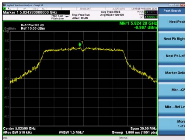
(802.11a) PSD plot on channel 165
