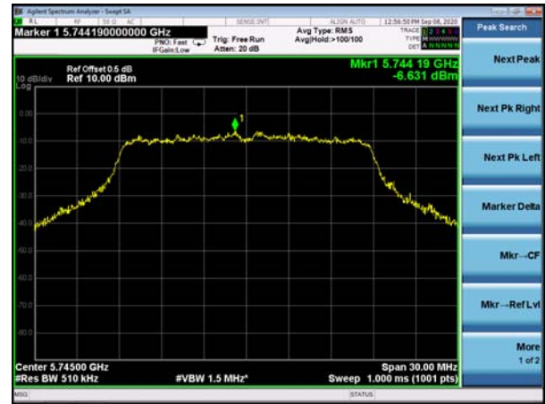
(802.11n20) PSD plot on channel 157
