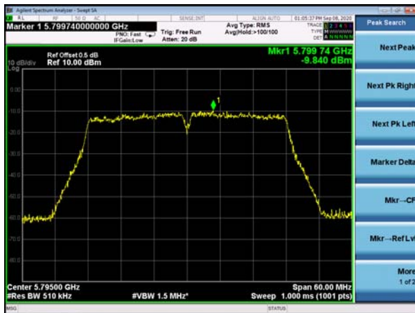
(802.11ac40) PSD plot on channel 159
