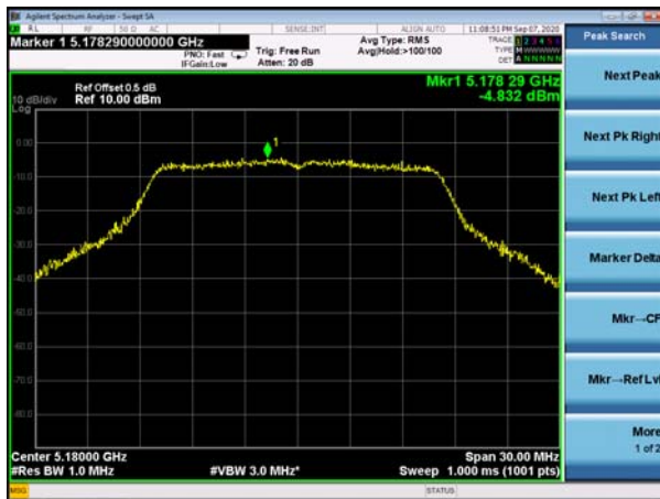
(802.11a) PSD plot on channel 40
