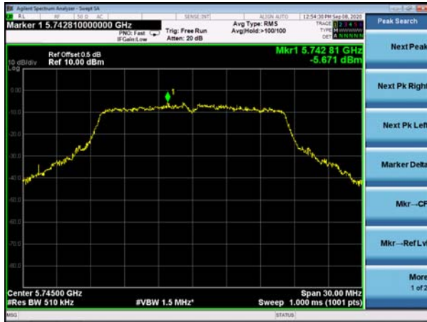
(802.11a) PSD plot on channel 157
