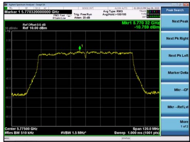
(802.11ac80) PSD plot on channel 155
