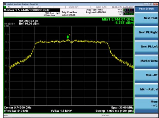
(802.11ac20) PSD plot on channel 157
