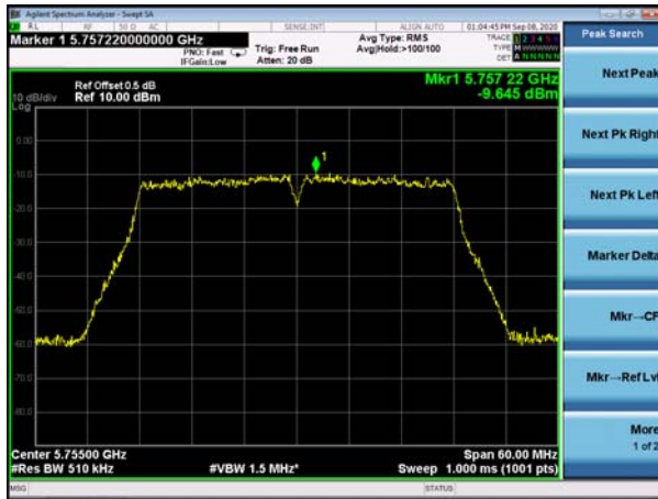
(802.11ac40) PSD plot on channel 159
