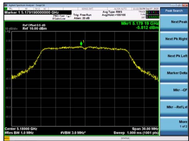
(802.11n20) PSD plot on channel 40
