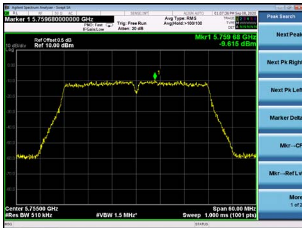
(802.11n40) PSD plot on channel 159
