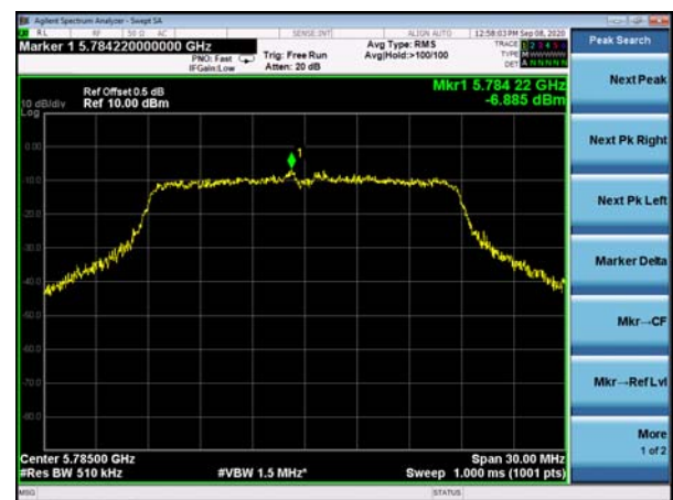
(802.11n20) PSD plot on channel 157
