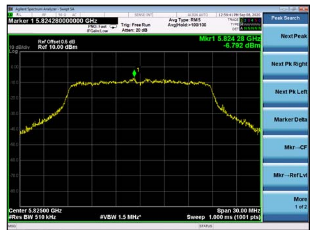
(802.11n20) PSD plot on channel 165
