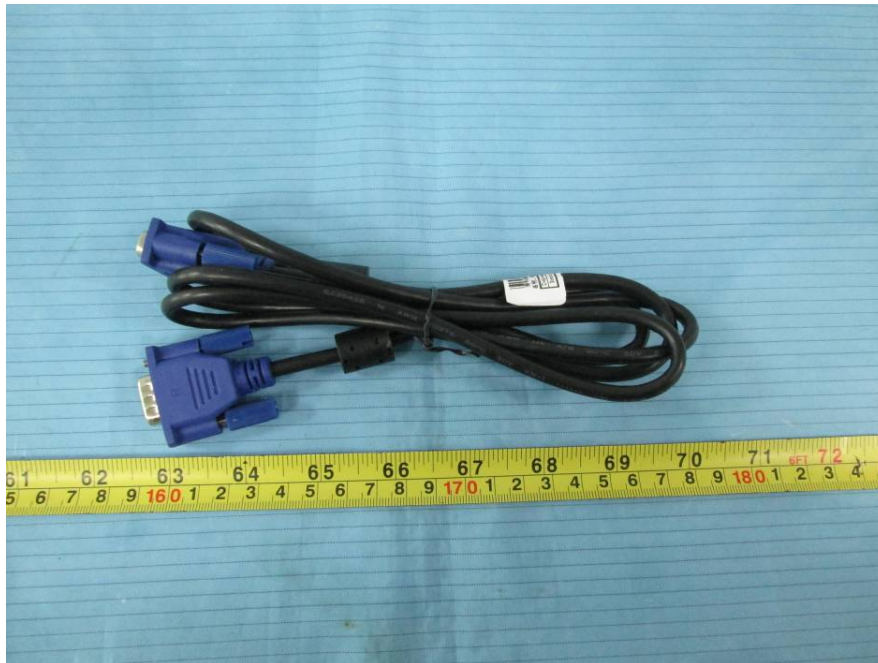
EUT – VGA Cable View
