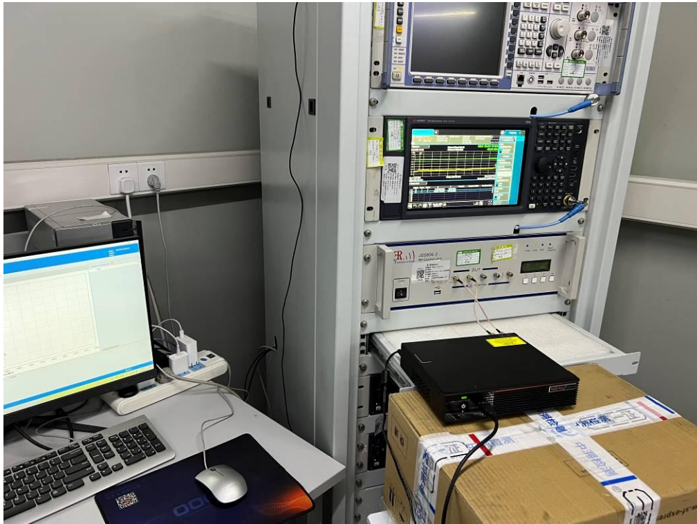
Description: Conducted Test Setup
