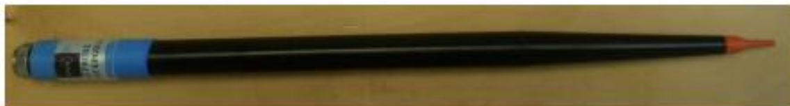
Figure 1 – MVG COMOSAR Dosimetric E field Dipole
