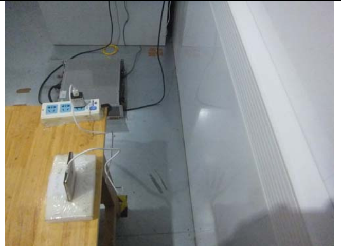
Conducted Emissions Test Setup Side View
