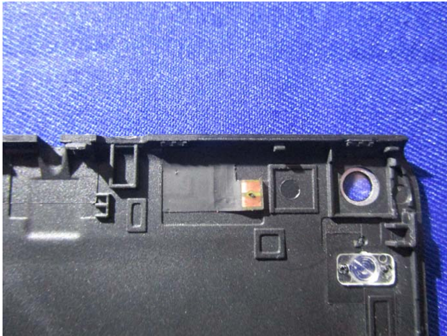
EUT – LTE Receive Antenna View
